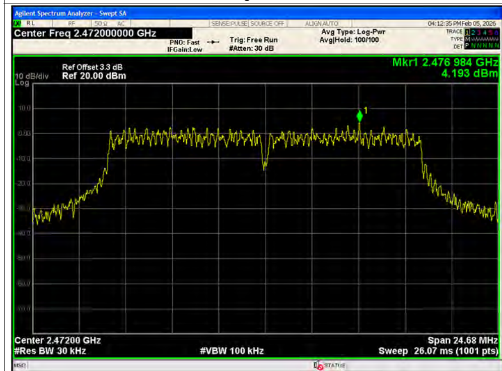
PSD NVNT g 2472MHz Ant1
