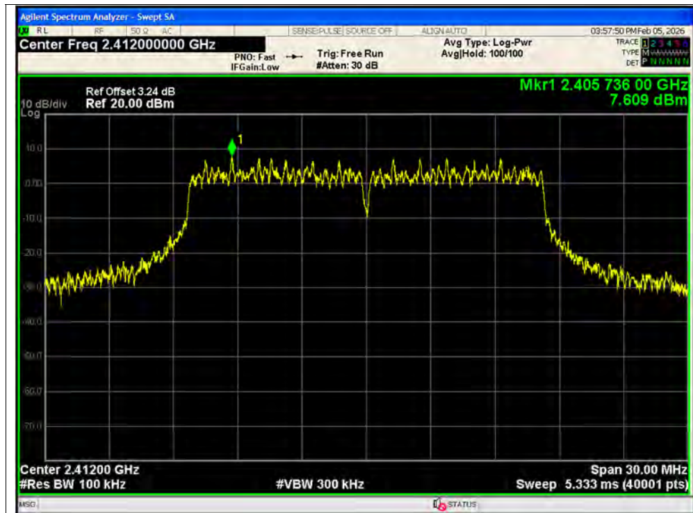
Tx. Spurious NVNT g 2412MHz Ant1 Ref
