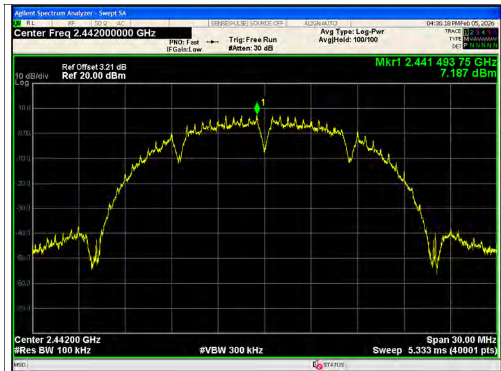
Tx. Spurious NVNT b 2442MHz Ant1 Ref
