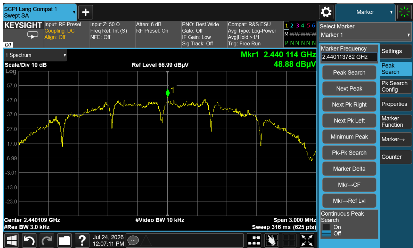
Figure 13: Power spectral Density - Middle Channel
