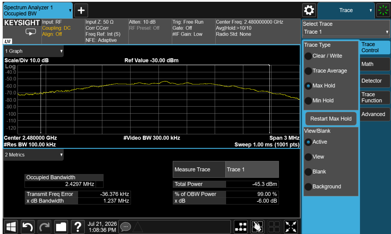
Figure 5: 6 dB Bandwidth - High Channel
