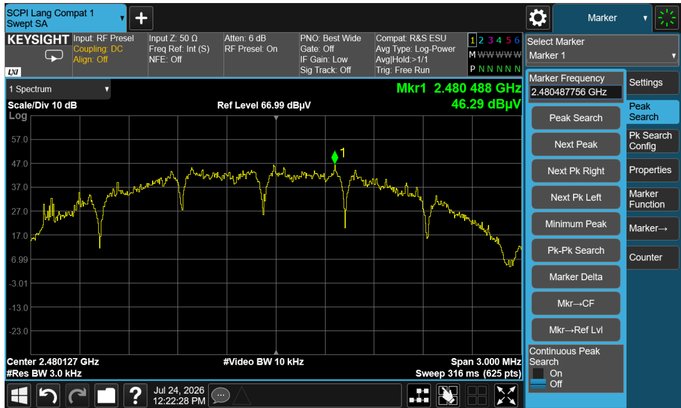
Figure 14: 99% Bandwidth - High Channel
