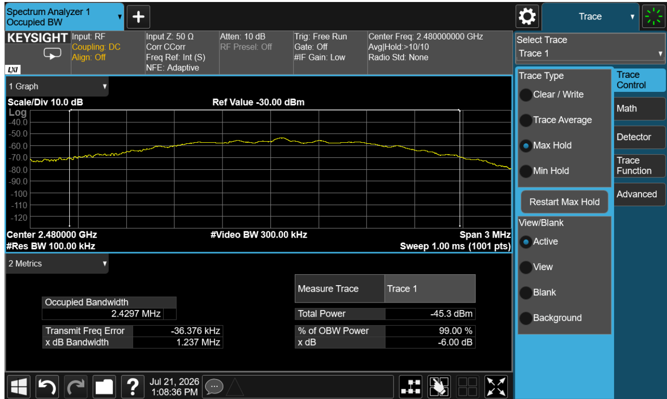
Figure 8: 99% Bandwidth - High Channel
