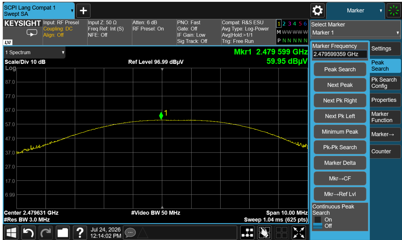
Figure 11: Peak Output Power - High Channel
