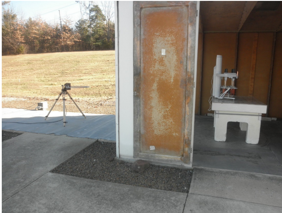
Antenna Parallel to Ground, Below 30 MHz
