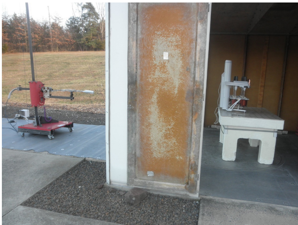
Horizontal Antenna Polarization, 200 MHz to 1 GHz
