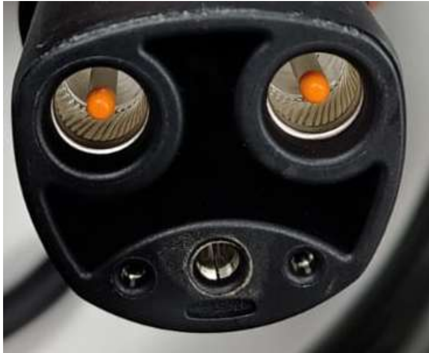
NACS Charging Gun/ Connector View
