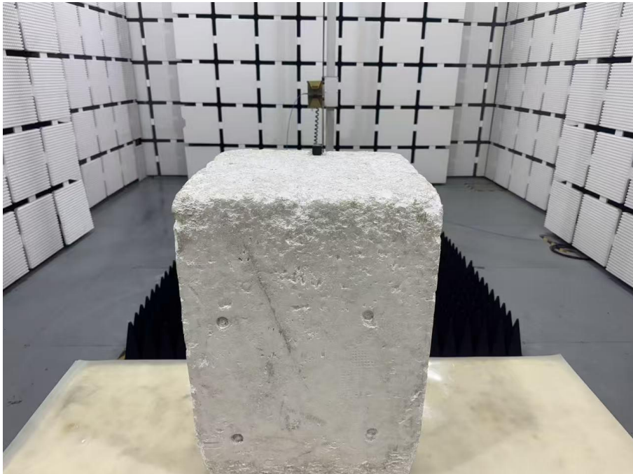
Set-up for Radiated Spurious Emission, Above 1GHz
