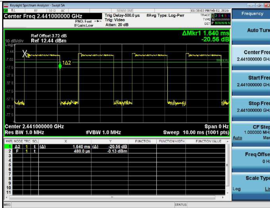
Dwell Time (Hopping) NVNT_ANT1_3-DH3_2441_00_Accumulated
