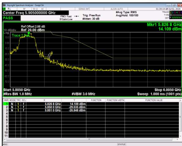
(802.11ac40 MIMO) Band Edge, Right Side
