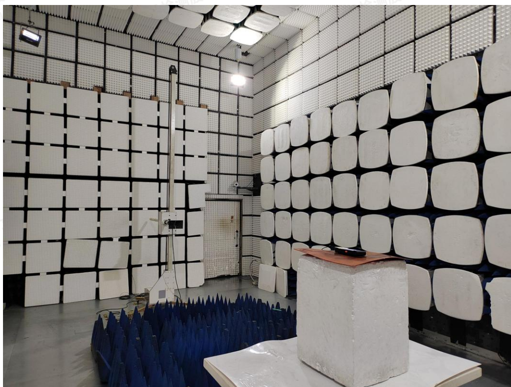
Radiated Emissions Measurement (Above 1GHz)
