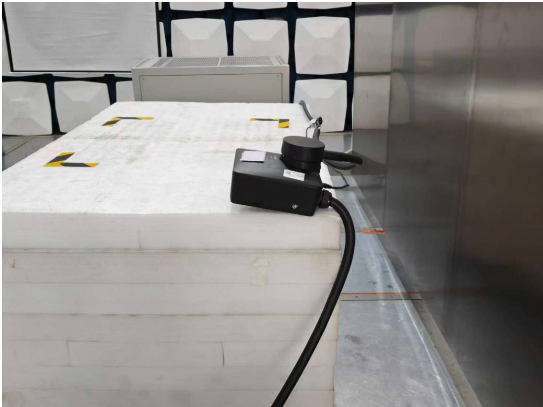
Conducted Emissions Side View
