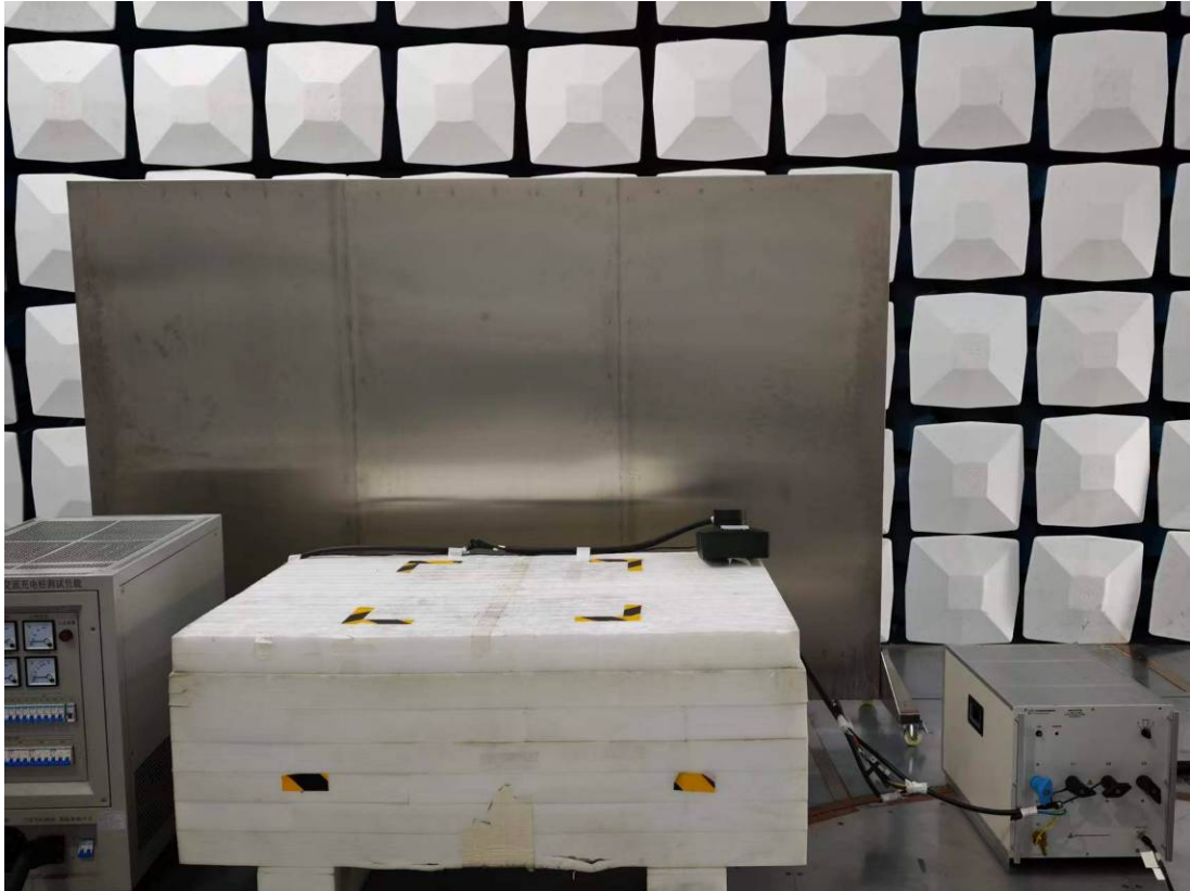
Conducted Emissions Side View
