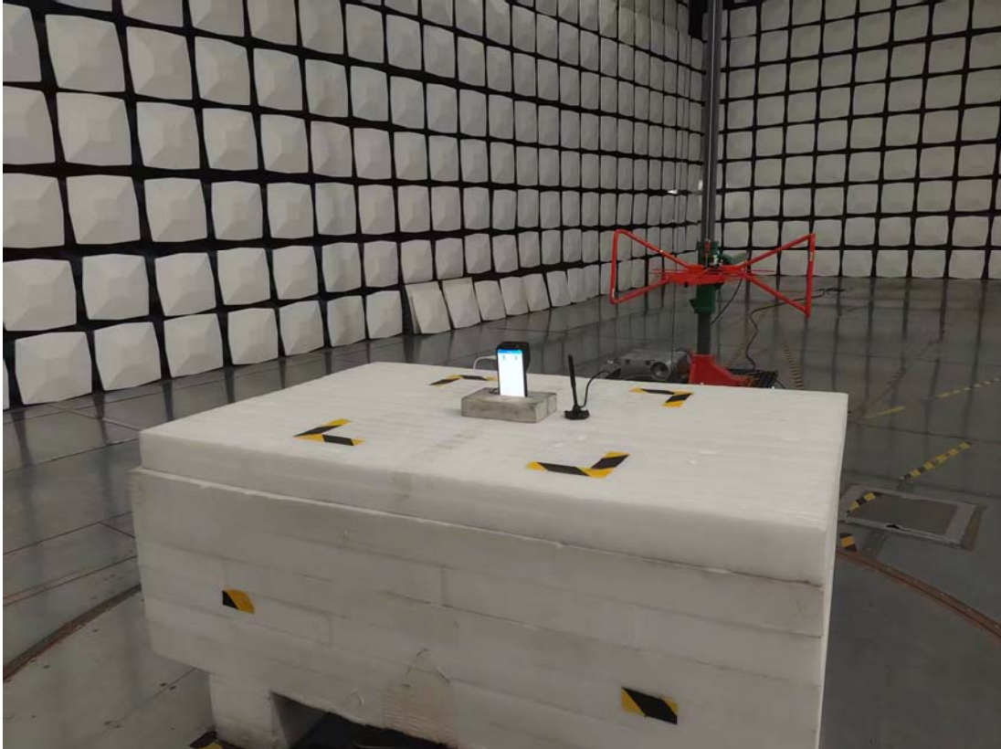
Radiated Emission 1-18GHz View
