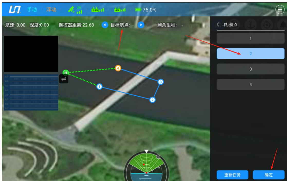
Figure 3-8 Target Waypoint Settings
