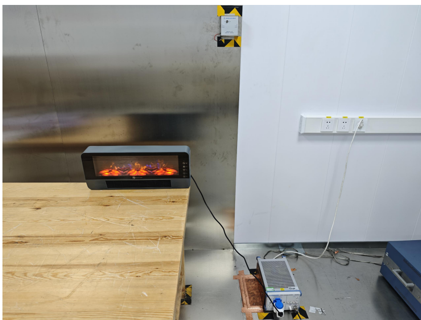
Conducted Emission Test View
