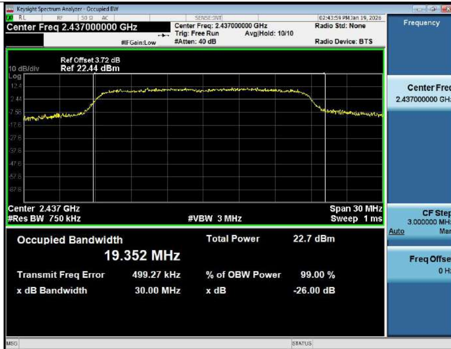
99% Occupied Bandwidth_NVNT_ANT1_802_11n(HT20)_2462
