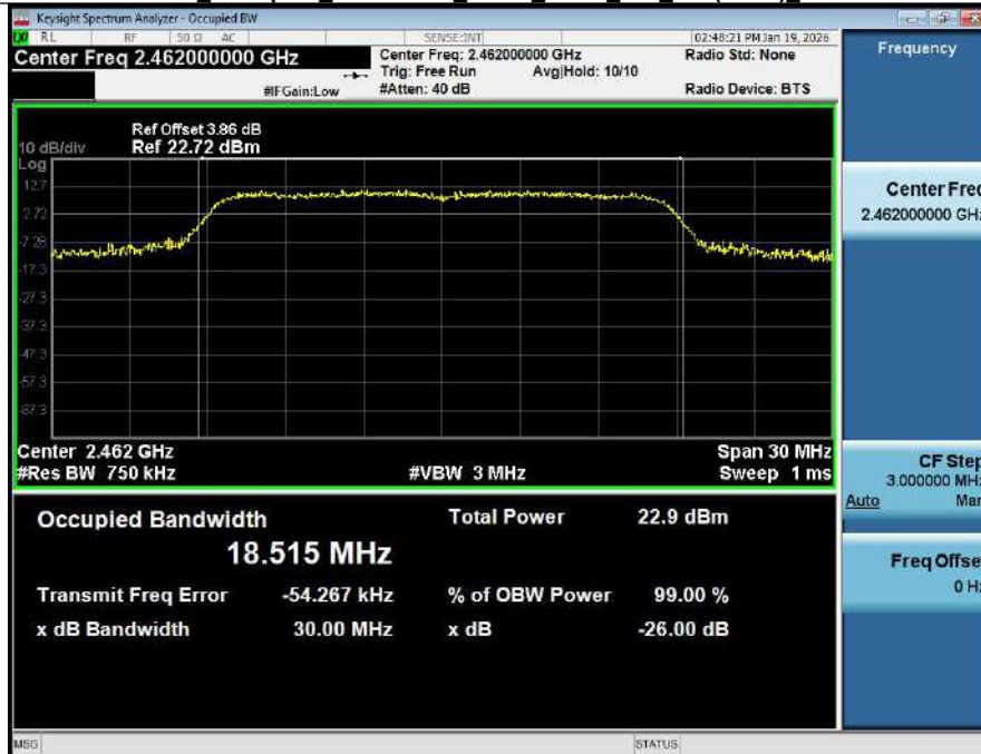
99% Occupied Bandwidth_NVNT_ANT1_802_11n(HT20)_2462
