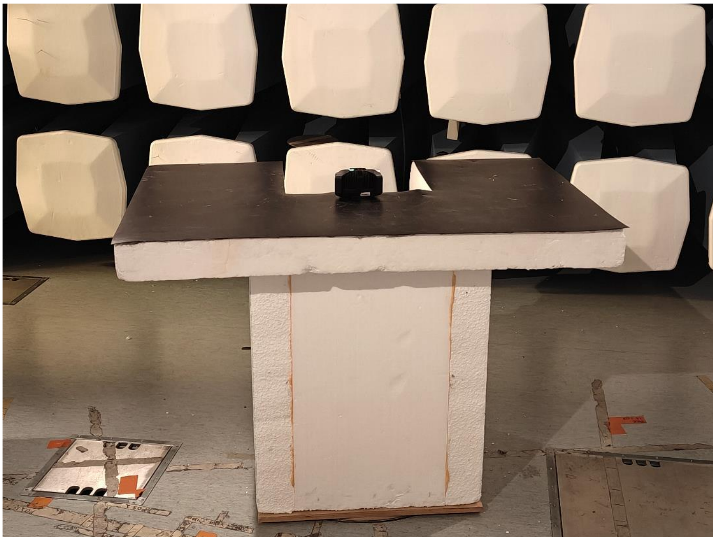
Picture 10 Radiated emission pictures 30-1000MHz
