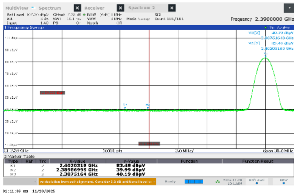
Figure 2.7.7-25 – Radiated Band-Edge Emissions Test Results – Vertical - Average
