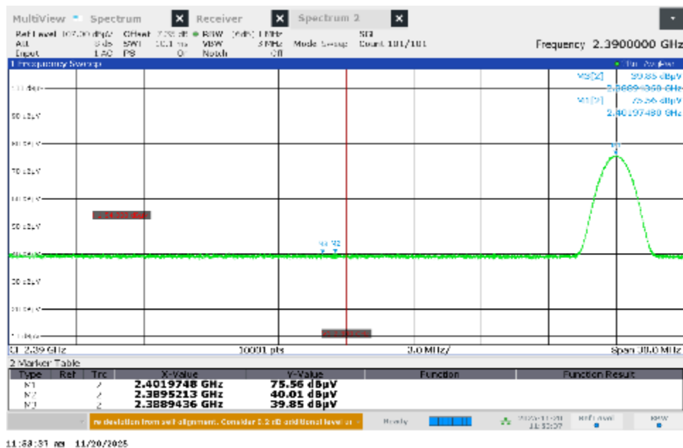
Figure 2.7.7-33 – Radiated Band-Edge Emissions Test Results – Horizontal - Average
