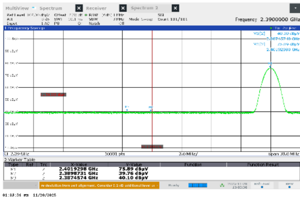
Figure 2.7.7-23 – Radiated Band-Edge Emissions Test Results – Horizontal - Average
