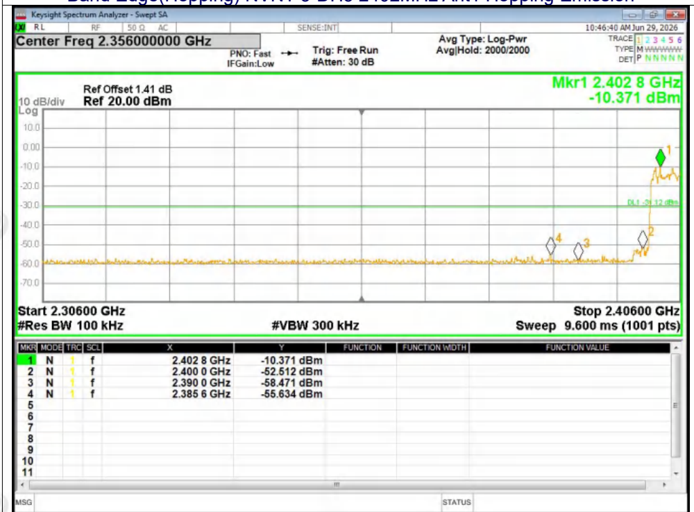
Band Edge(Hopping) NVNT 3-DH5 2402MHz Ant1 Hopping Emission
