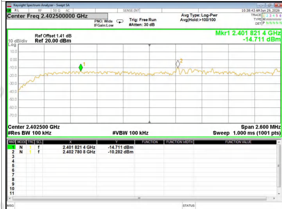
CFS NVNT 2-DH5 2402MHz Ant1
