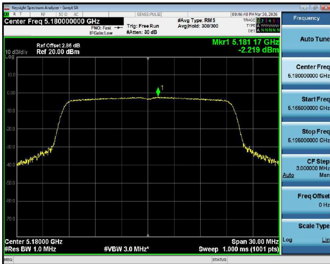
PSD NVNT ax20 5180MHz Ant1
