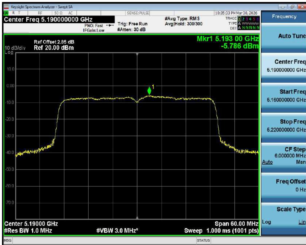
PSD NVNT ax40 5190MHz Ant1
