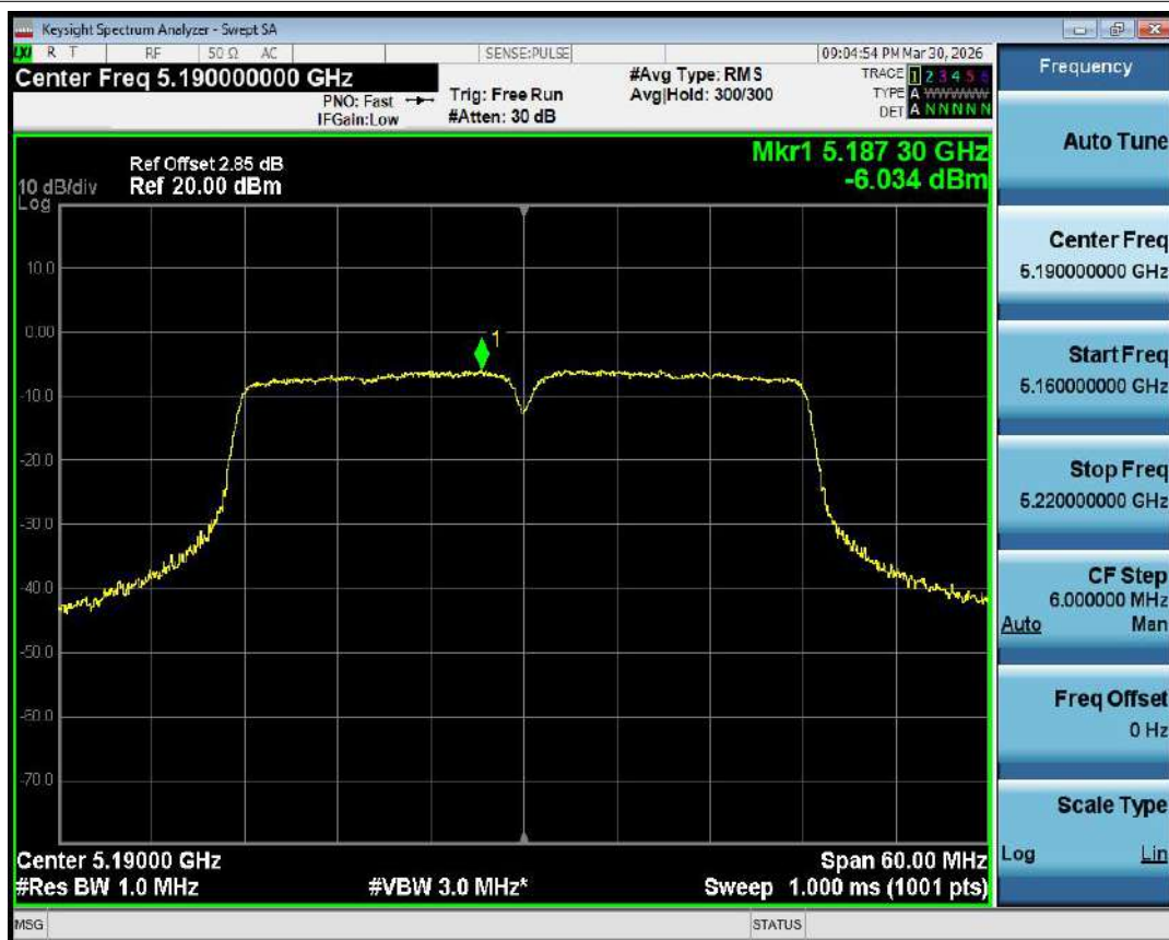
PSD NVNT ac40 5190MHz Ant1
