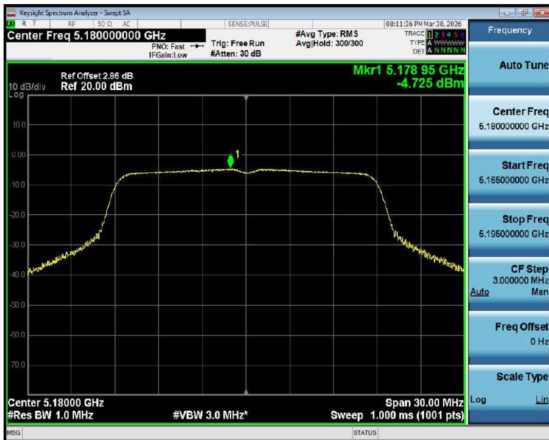
PSD NVNT n20 5180MHz Ant1
