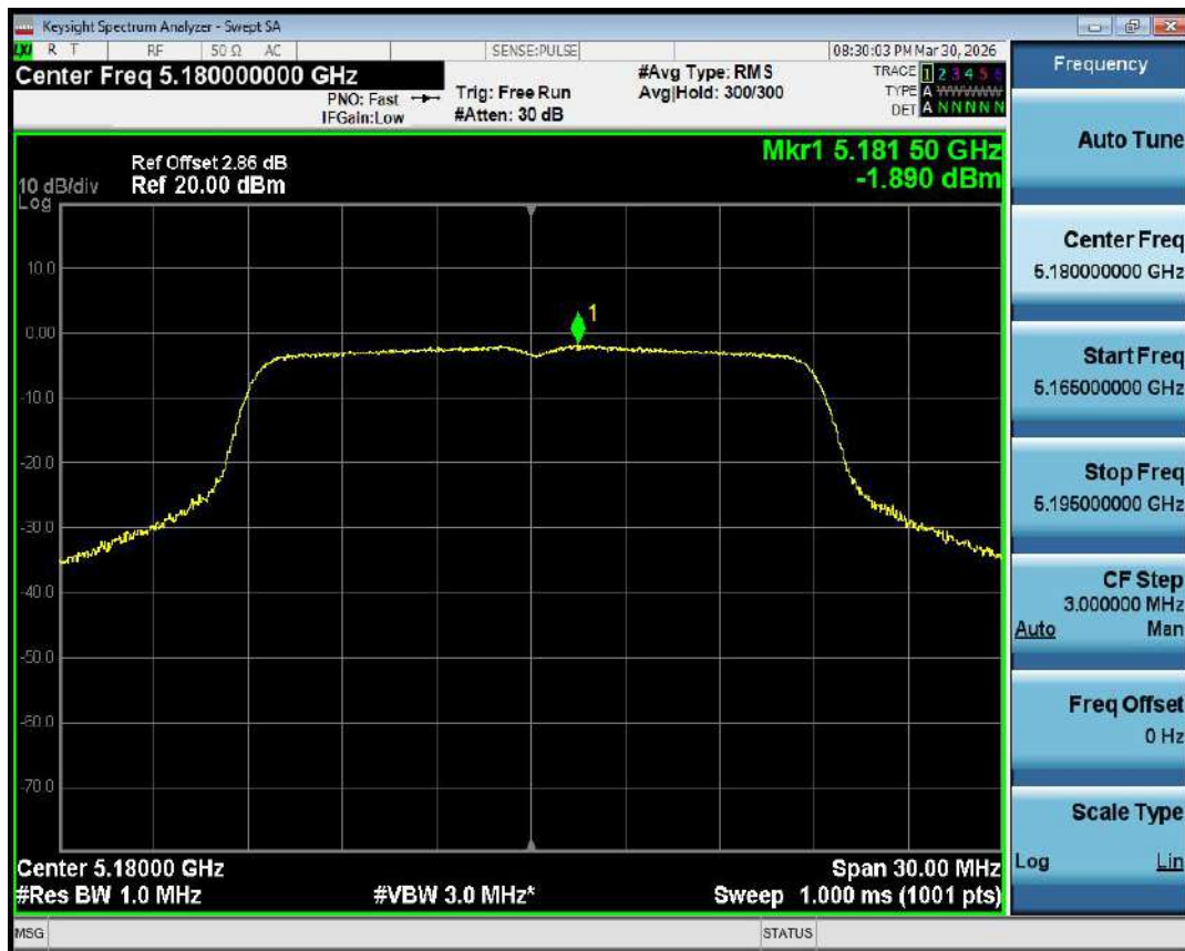
PSD NVNT ac20 5180MHz Ant1
