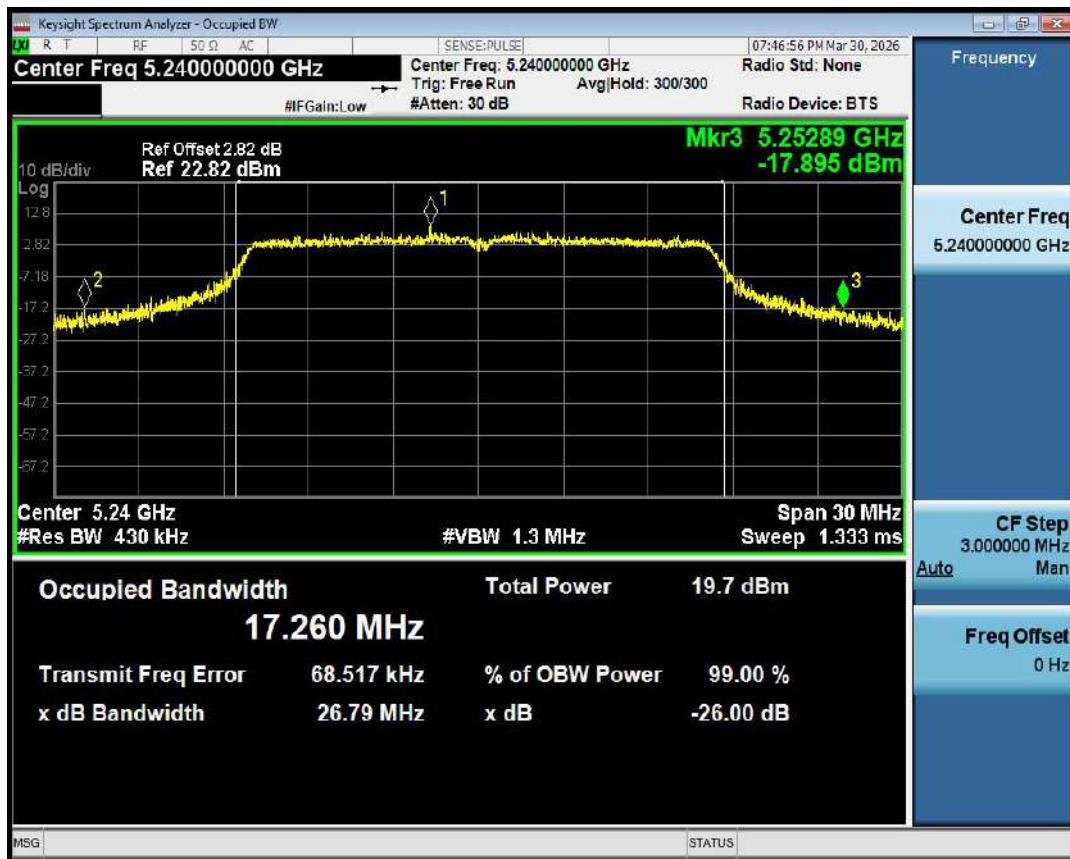
-26dB Bandwidth NVNT a 5240MHz Ant1
