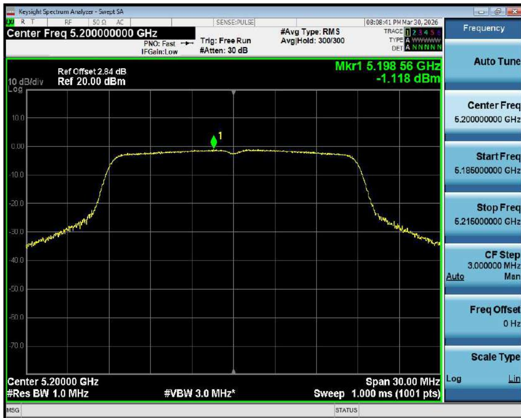
PSD NVNT n20 5200MHz Ant1
