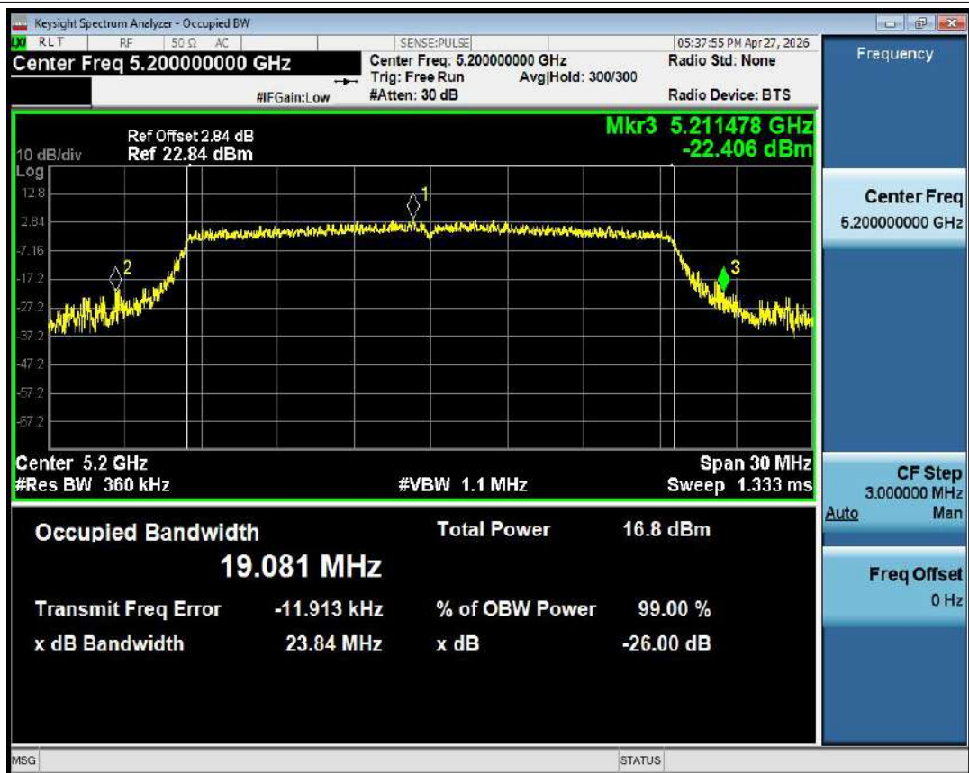
-26dB Bandwidth NVNT ax20 5200MHz Ant1
