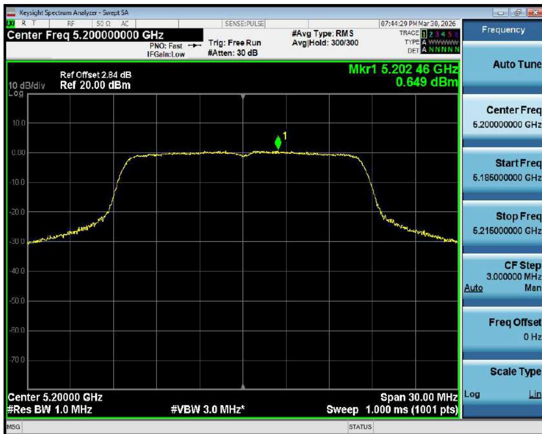
PSD NVNT a 5200MHz Ant1
