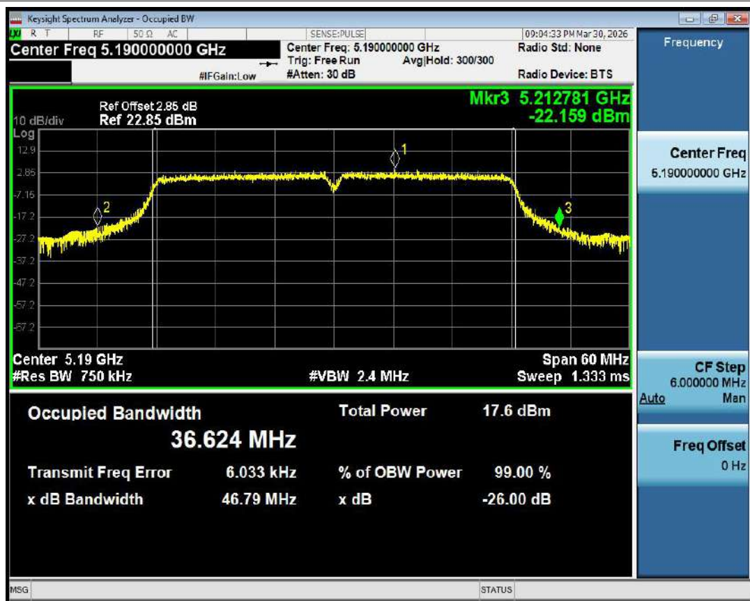
-26dB Bandwidth NVNT ac40 5190MHz Ant1
