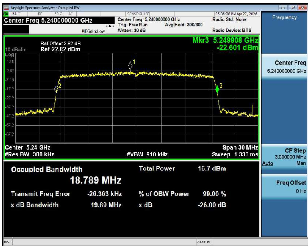
-26dB Bandwidth NVNT ax20 5240MHz Ant1
