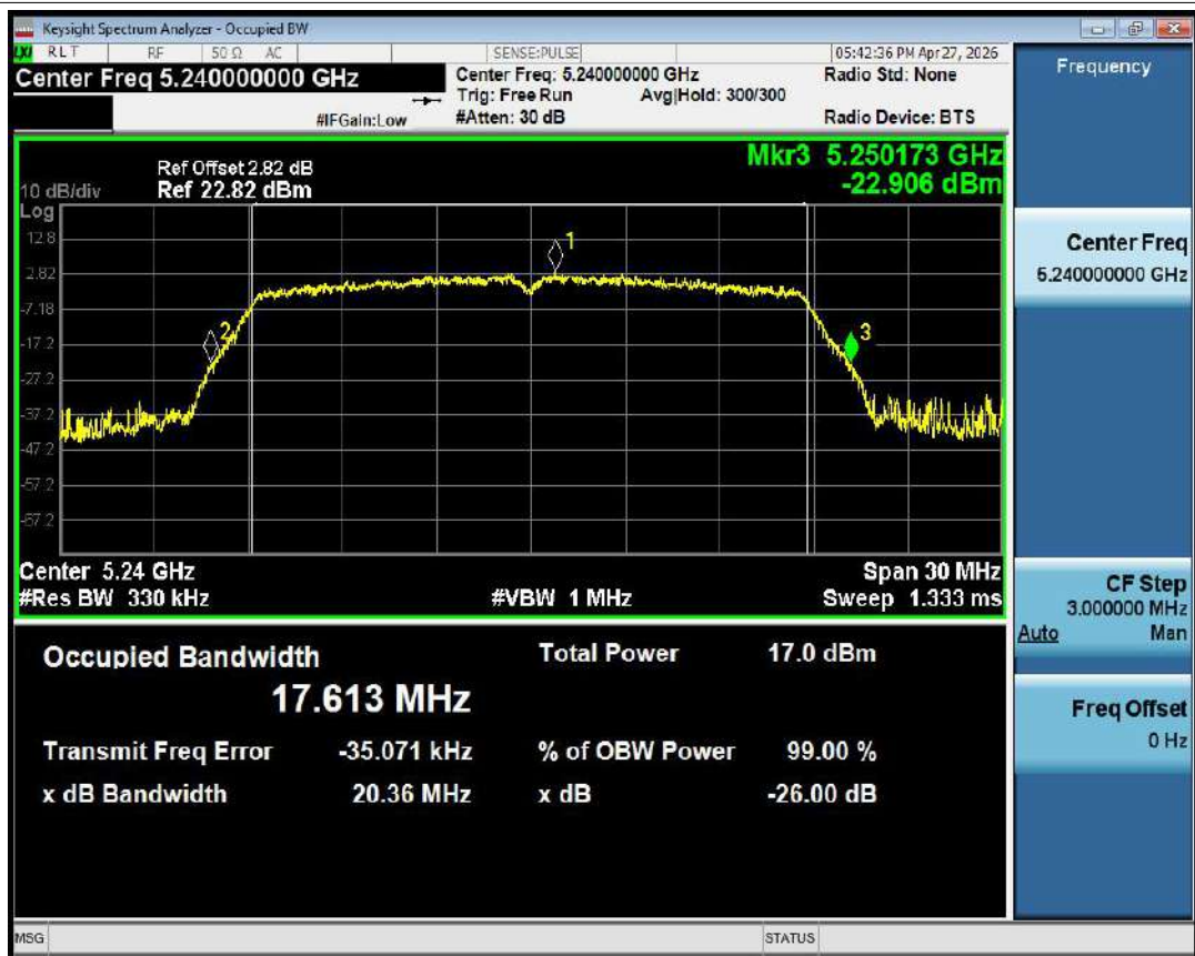
-26dB Bandwidth NVNT ac20 5240MHz Ant1
