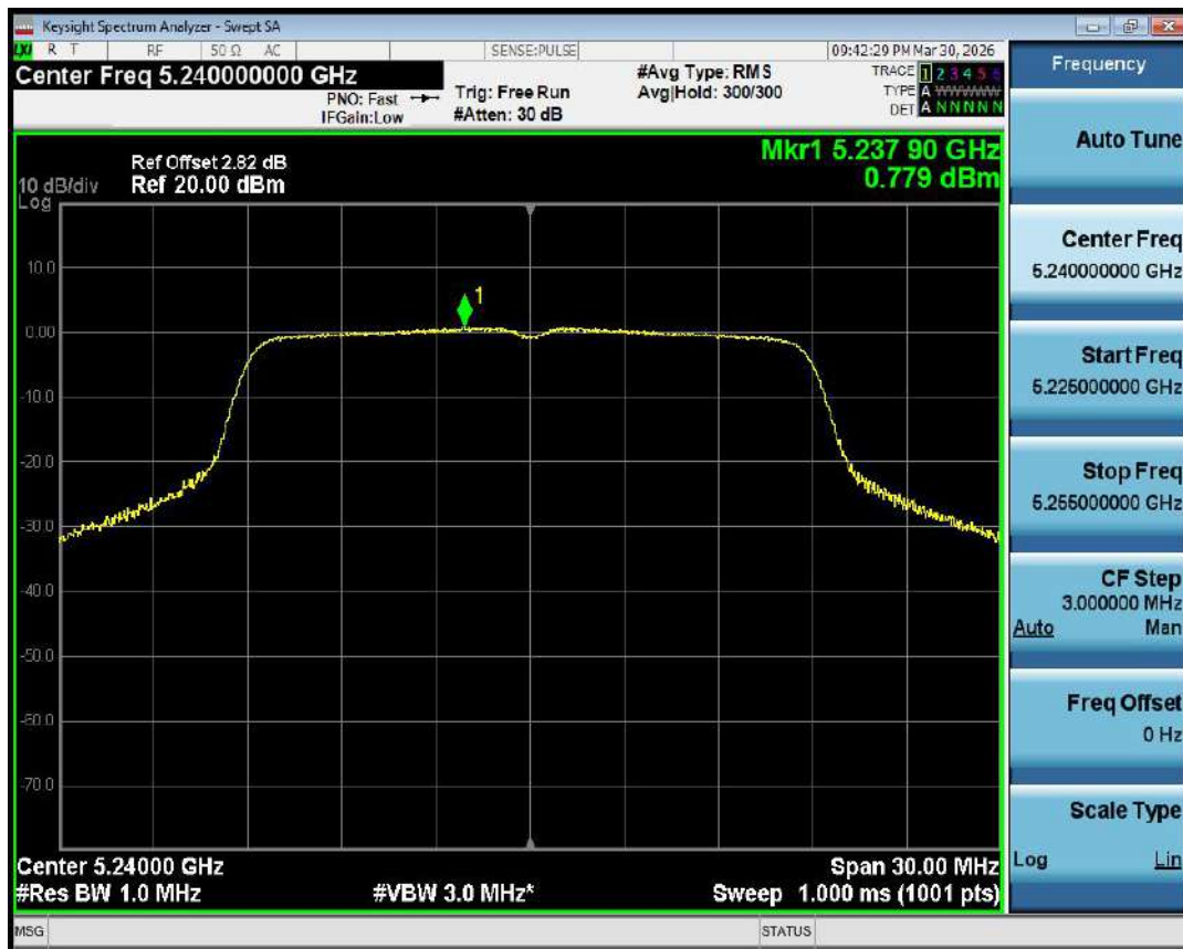
PSD NVNT ac20 5240MHz Ant1
