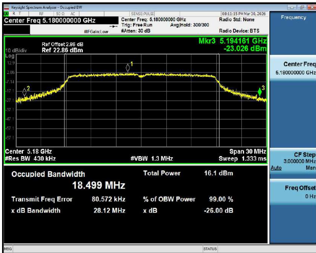
-26dB Bandwidth NVNT n20 5180MHz Ant1
