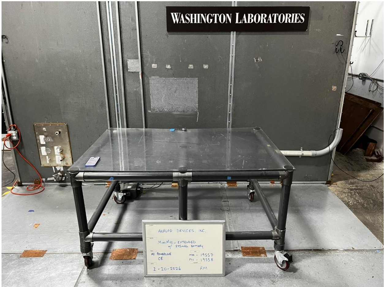
AC Powerline Conducted Emissions, View 1
