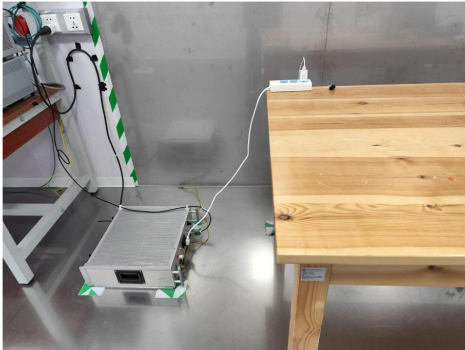
Conducted Emission at AC power line
