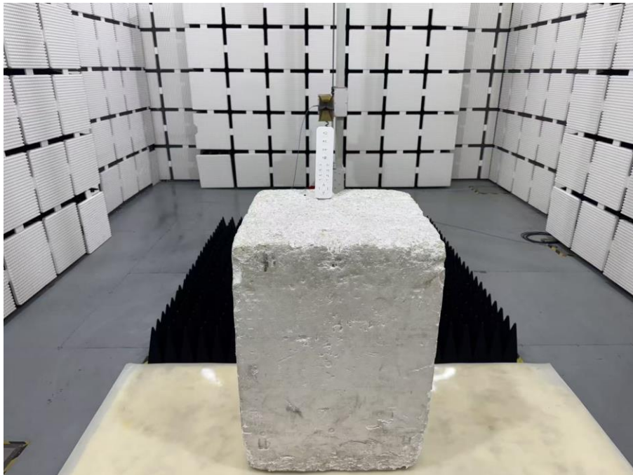
Set-up for Radiated Spurious Emission, Above 1GHz
