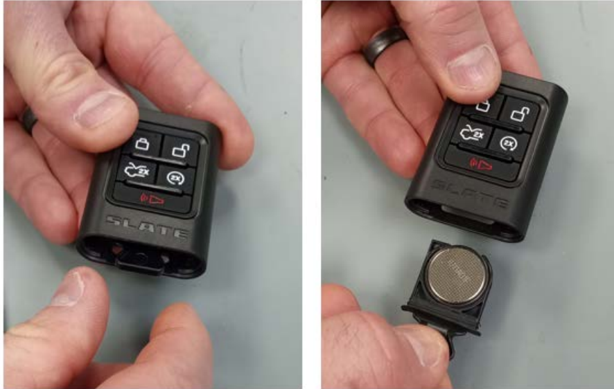
Figure 4. Removal of the battery tray with battery.
