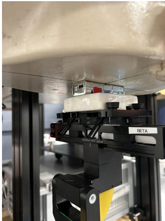
Figure 1 SAR Test Setup – Body/Extremity – Back Side 0mm
