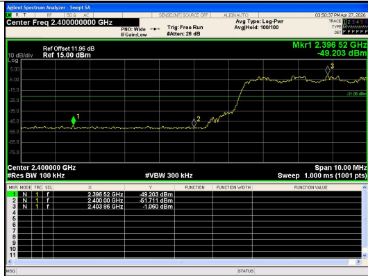
Out Of Band Emission(Left) \pi/4 DQPSK_2-DH5_Channel Hopping
