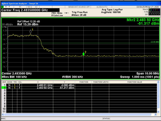
Out Of Band Emission(Right) 8DPSK_3-DH5_Channel Hopping
