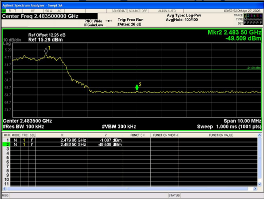
Out Of Band Emission(Right) 8DPSK_3-DH5_Channel Hopping
