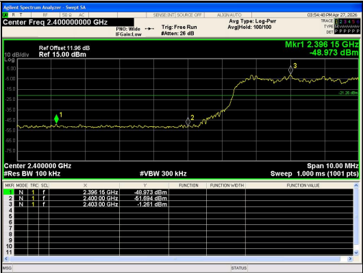
Out Of Band Emission(Left) 8DPSK_3-DH5_Channel Hopping
