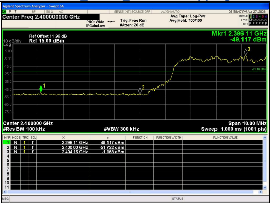
Out Of Band Emission(Left) 8DPSK_3-DH5_Channel Hopping
