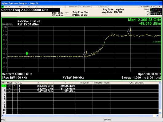
Out Of Band Emission(Left) 8DPSK_3-DH5_Channel Hopping
