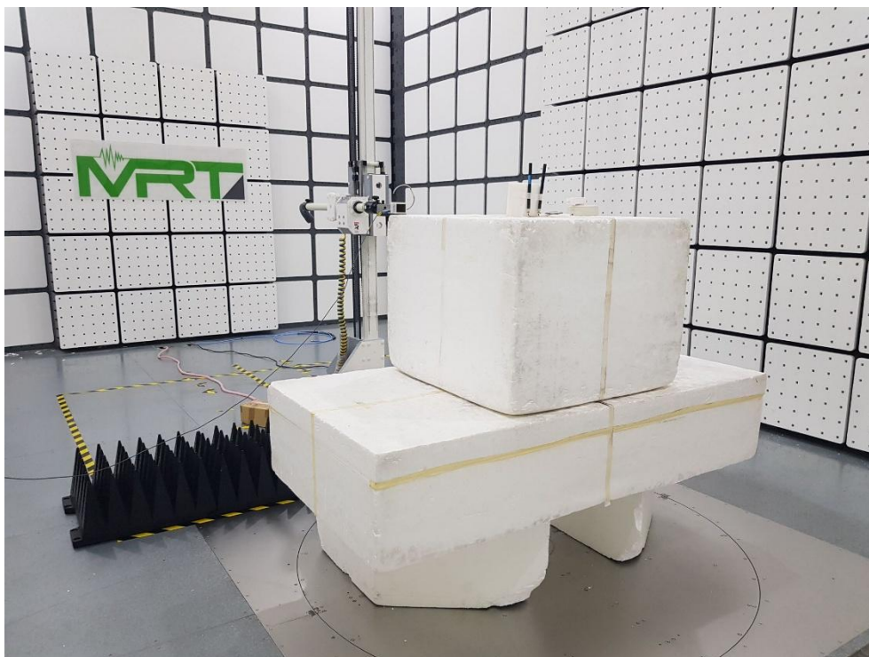
Description: Radiated Emission Test Setup for 18GHz~40GHz
