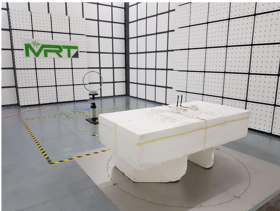
Description: Radiated Emission Test Setup for 18GHz~40GHz
