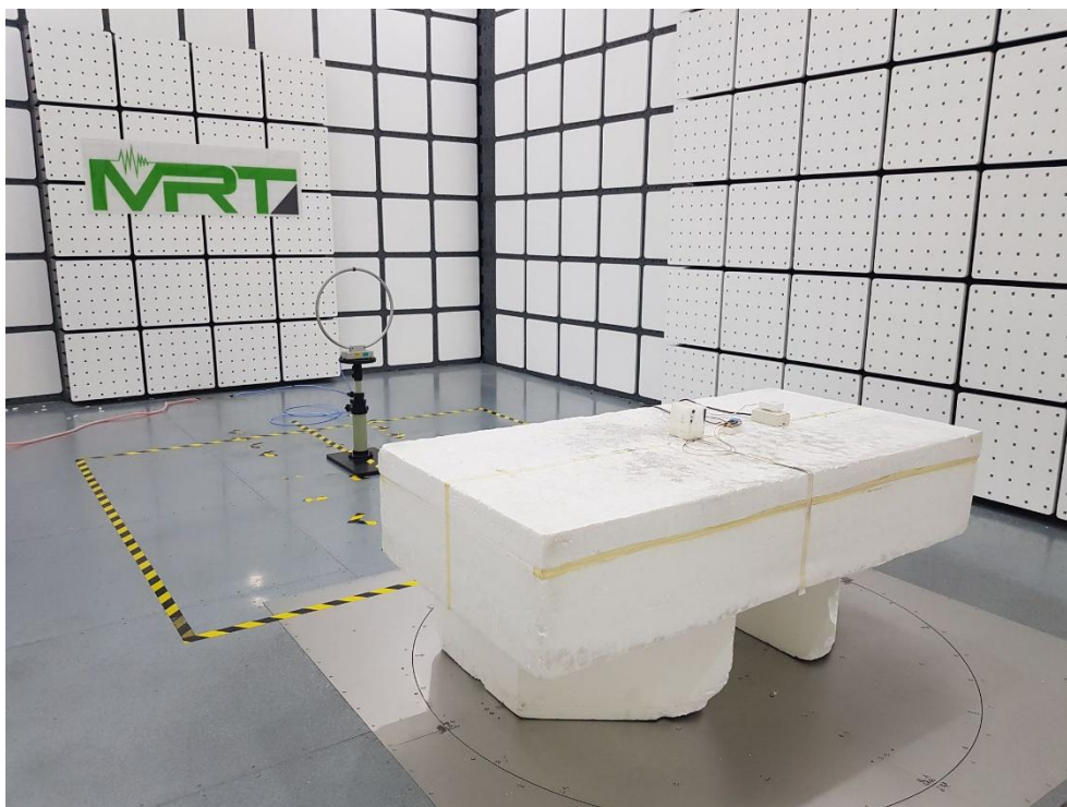
Description: Radiated Emission Test Setup for 18GHz~40GHz
