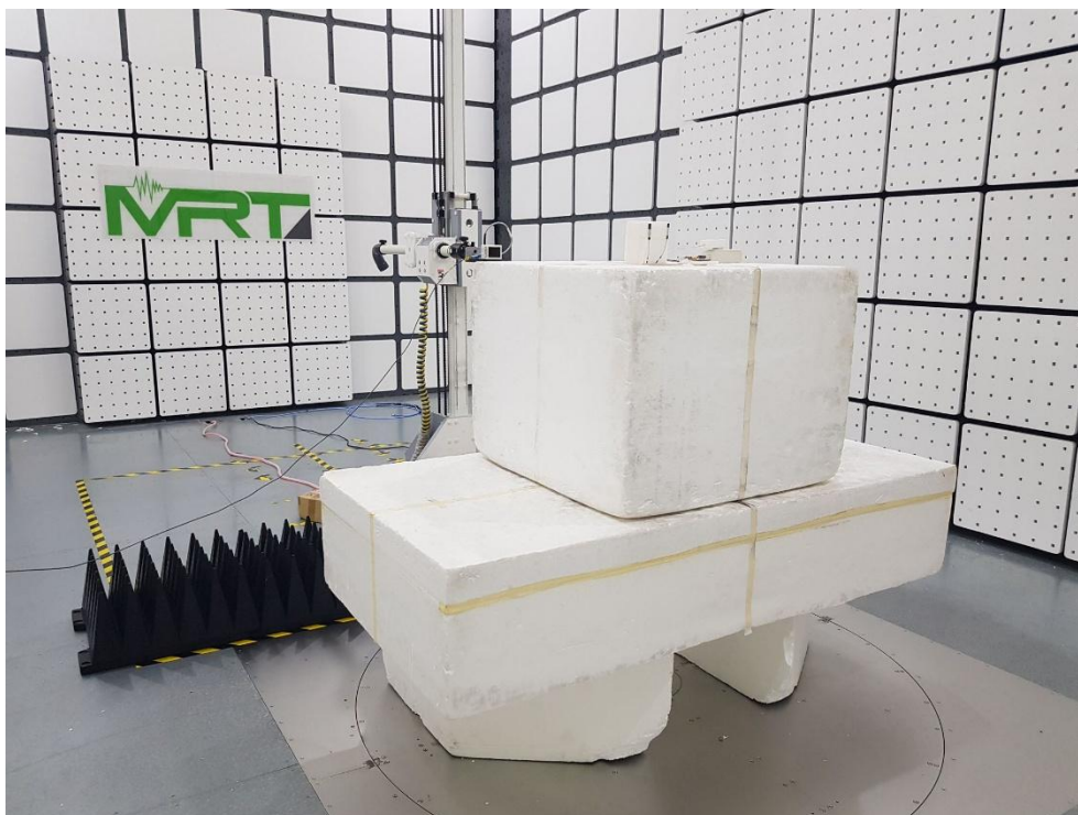
Description: Radiated Emission Test Setup for 18GHz~40GHz
