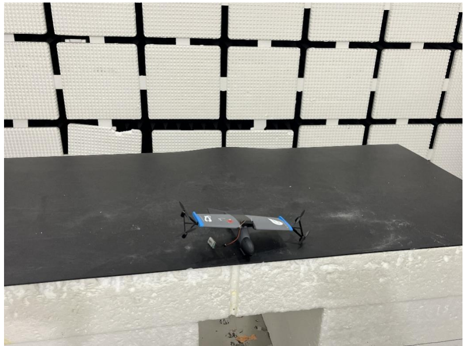
Radiation Emission Test Setup (close up)
