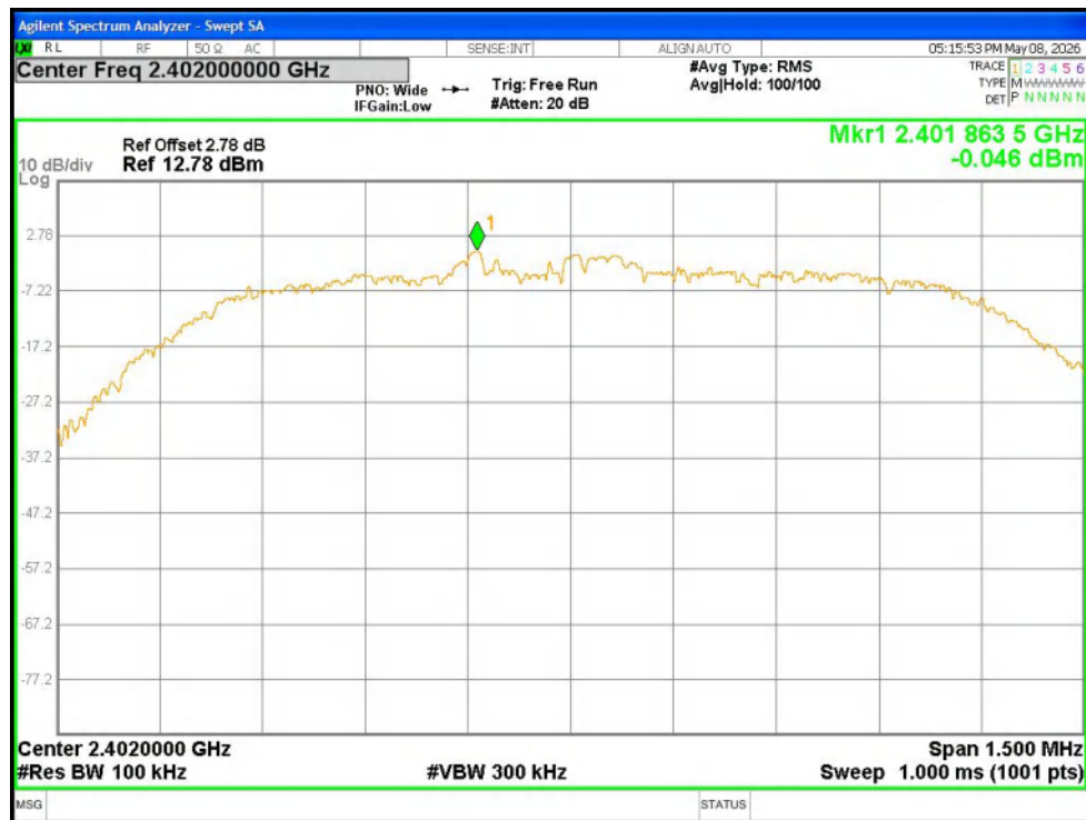
Tx. Spurious NVNT 2-DH5 2402MHz Ant1 Ref
