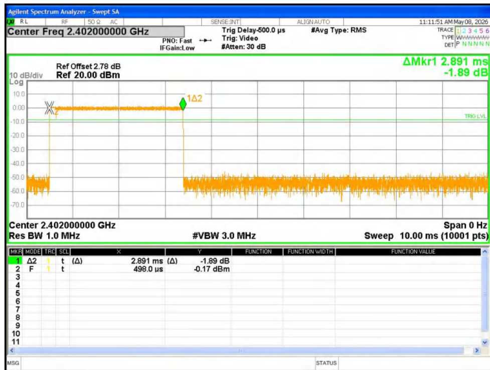
Dwell NVNT 2-DH5 2402MHz Ant1 One Burst
