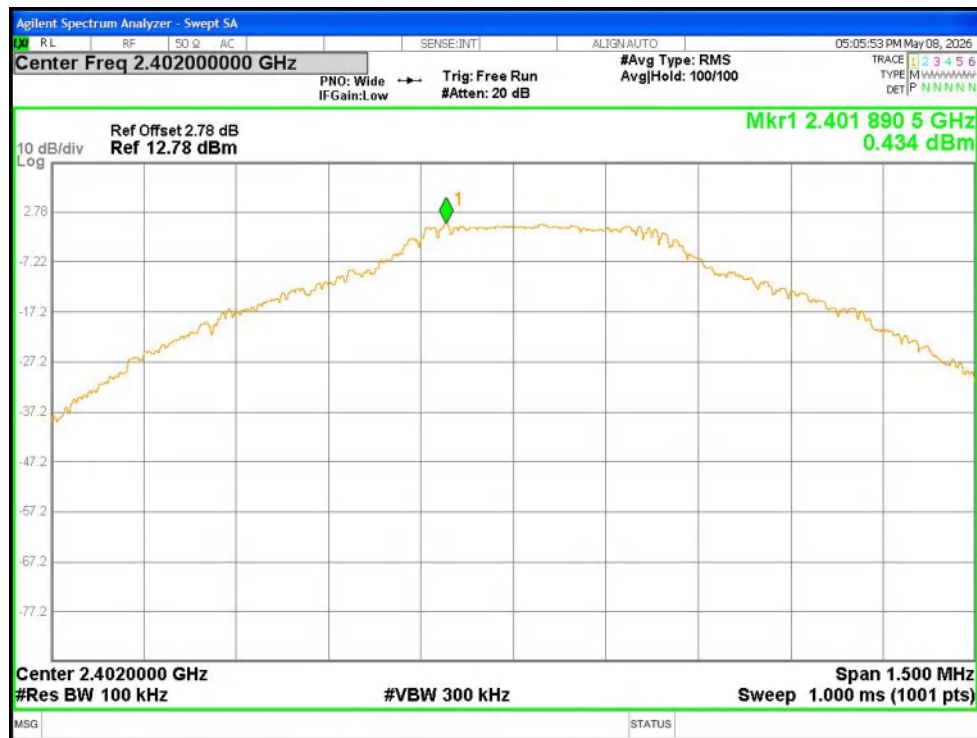
Tx. Spurious NVNT 1-DH5 2402MHz Ant1 Ref
