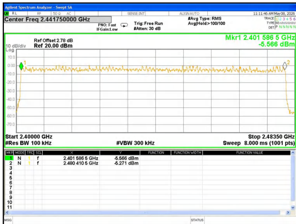
Hopping No. NVNT 2-DH5 2402MHz Ant1
