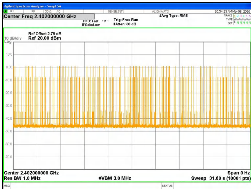
Dwell NVNT 1-DH5 2402MHz Ant1 Accumulated
