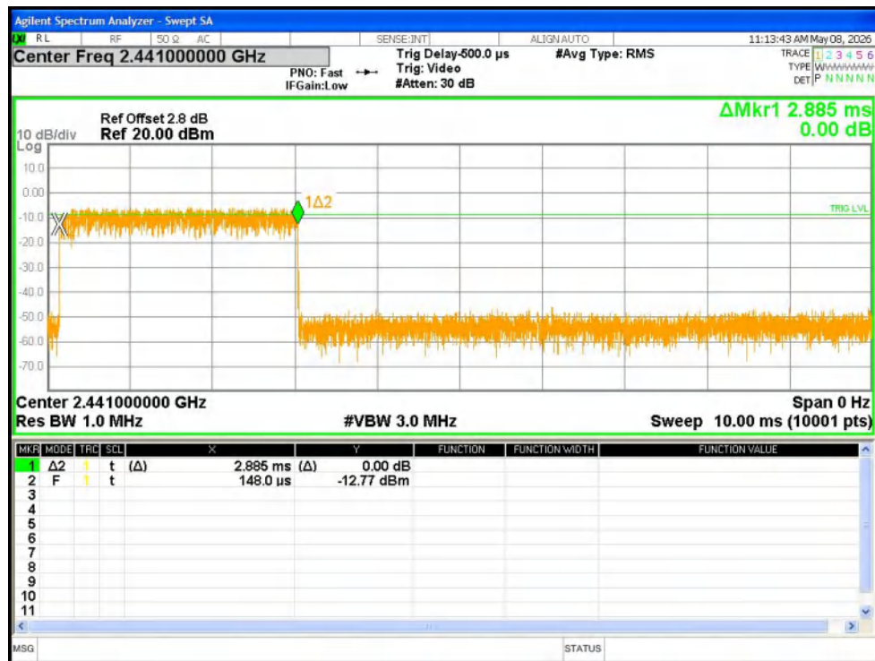
Dwell NVNT 2-DH5 2441MHz Ant1 One Burst
