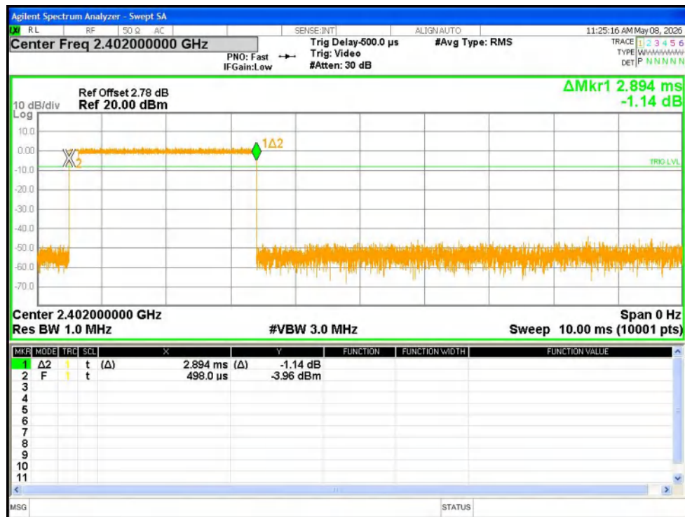
Dwell NVNT 3-DH5 2402MHz Ant1 One Burst
