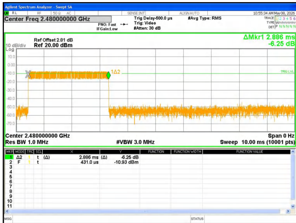
Dwell NVNT 1-DH5 2480MHz Ant1 One Burst
