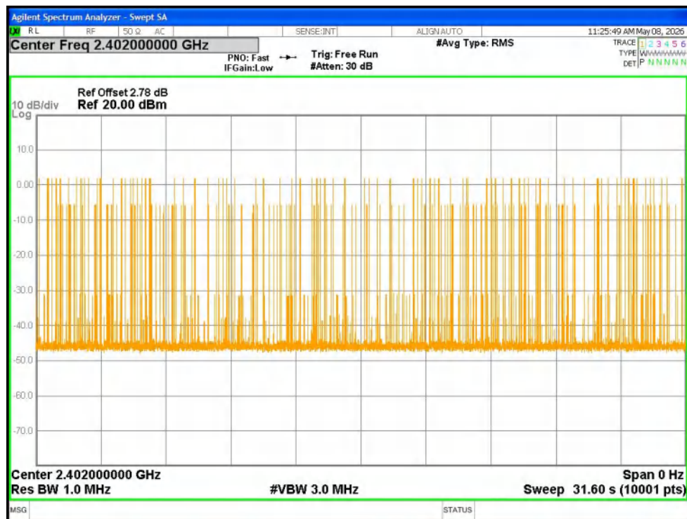
Dwell NVNT 3-DH5 2402MHz Ant1 Accumulated
