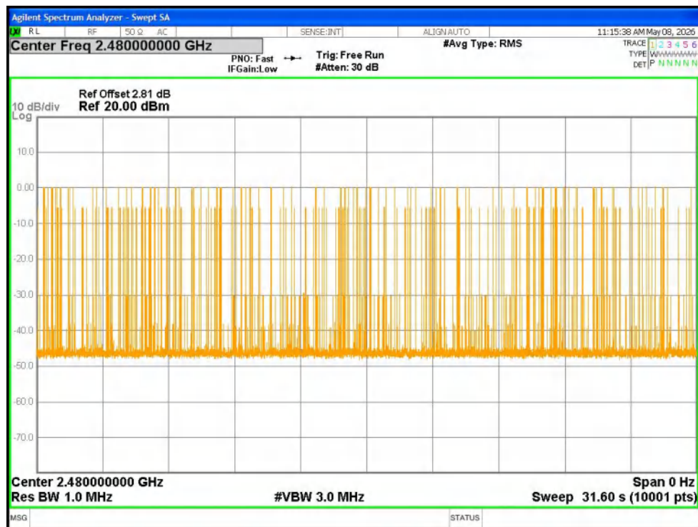
Dwell NVNT 2-DH5 2480MHz Ant1 Accumulated
