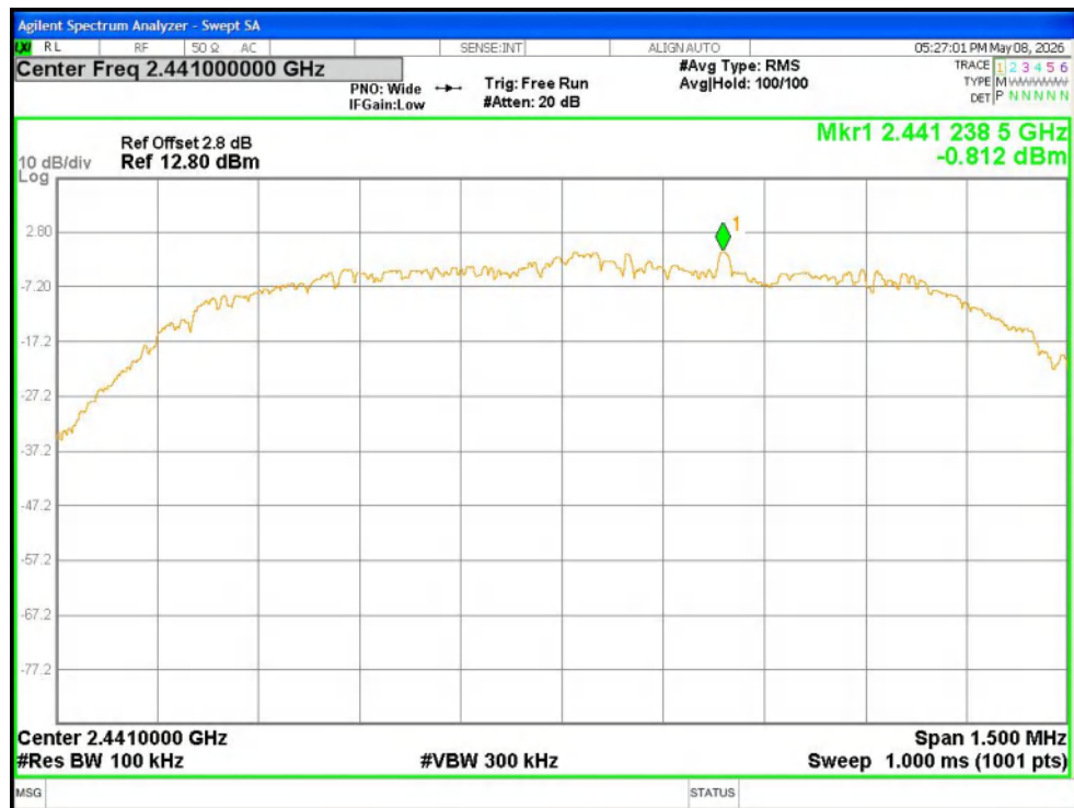
Tx. Spurious NVNT 3-DH5 2441MHz Ant1 Ref
