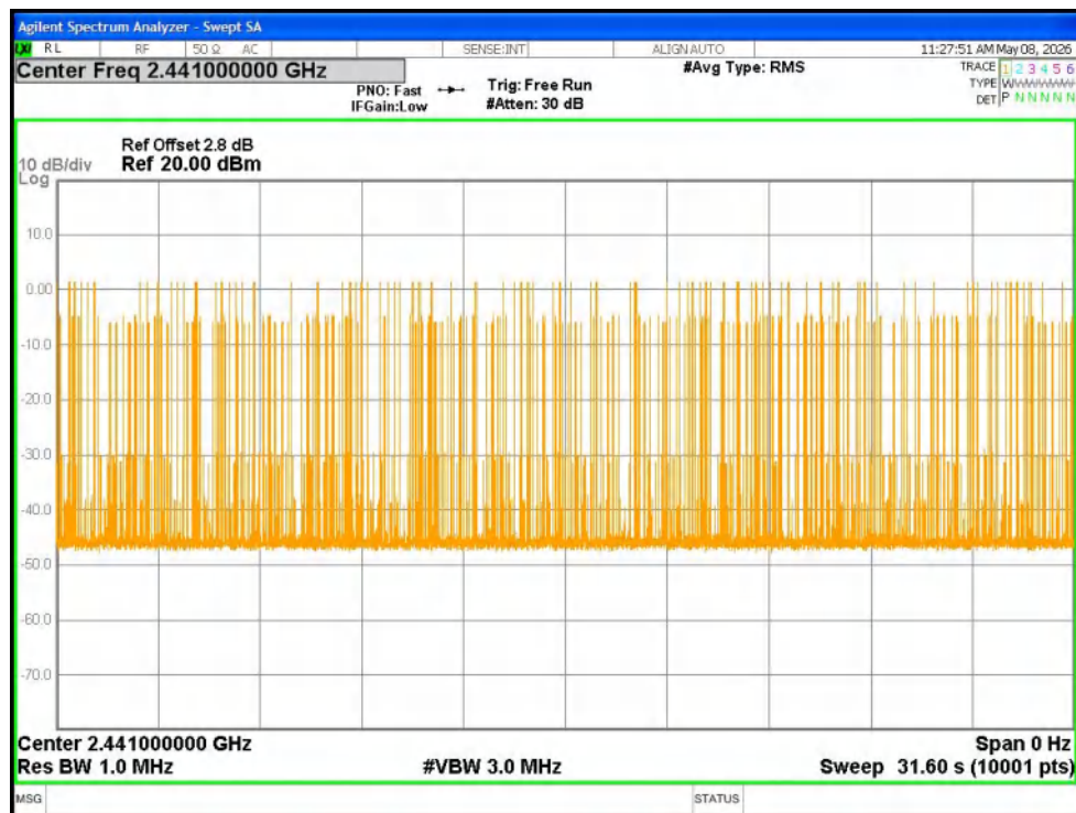
Dwell NVNT 3-DH5 2441MHz Ant1 Accumulated
