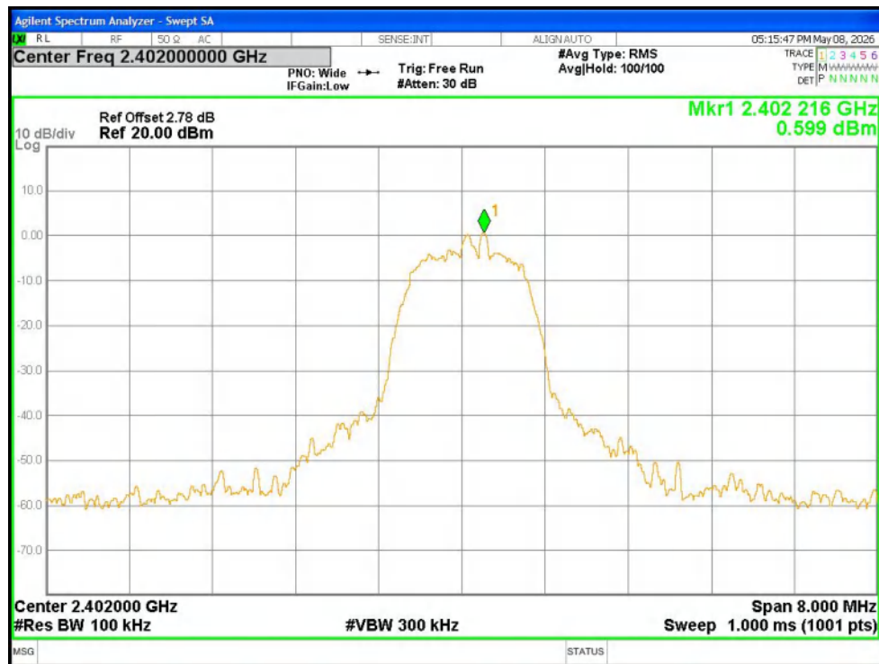
Band Edge NVNT 2-DH5 2402MHz Ant1 No-Hopping Ref
