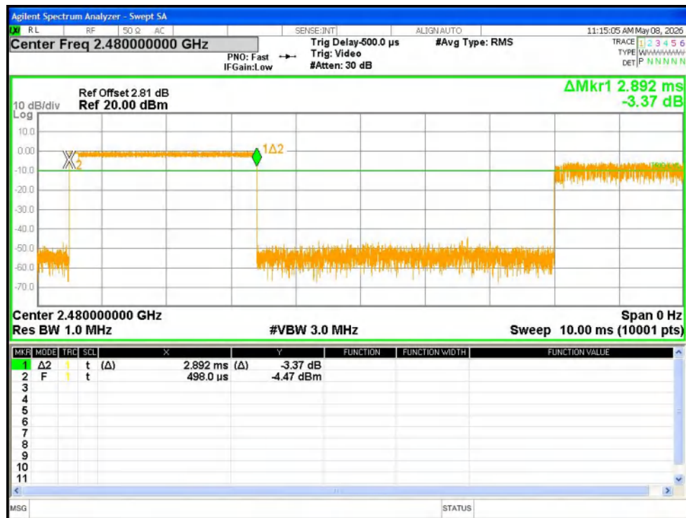
Dwell NVNT 2-DH5 2480MHz Ant1 One Burst
