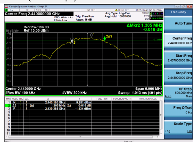
GFSK (BLE 2Mbps) LOW CHANNEL
