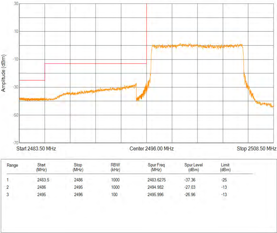
Band41 QPSK BW=10MHz Channel=41540 RB Size=1 Position=#0
