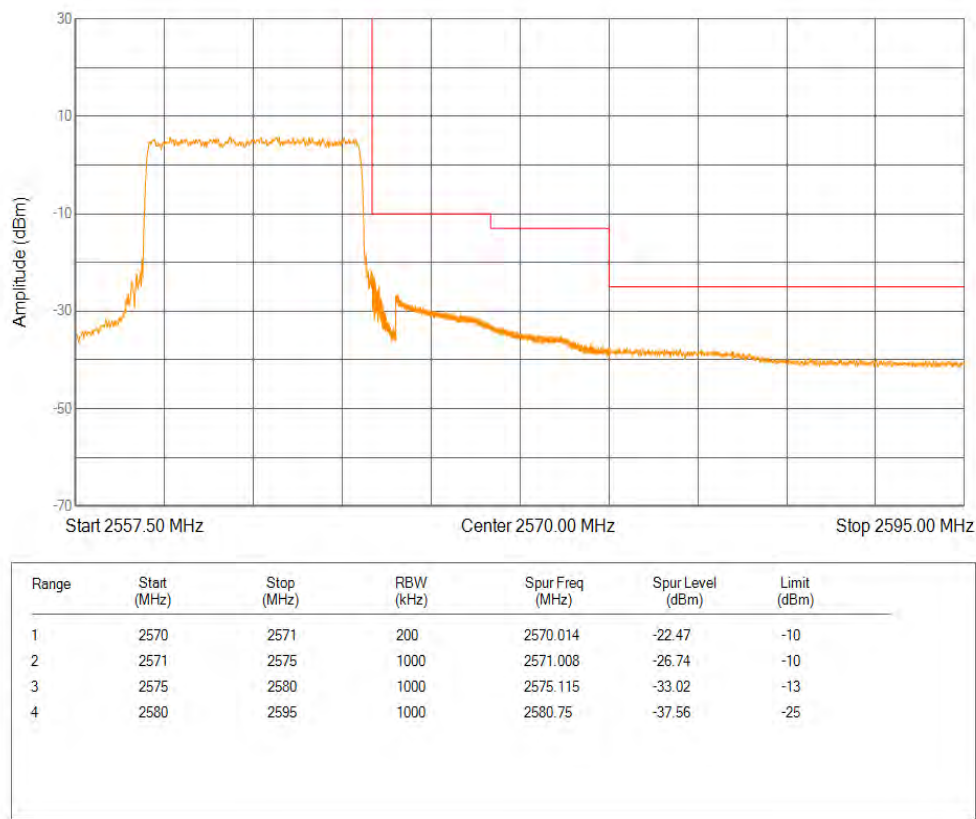
Band7 QPSK BW=15MHz Channel=20825 RB Size=1 Position=#0
