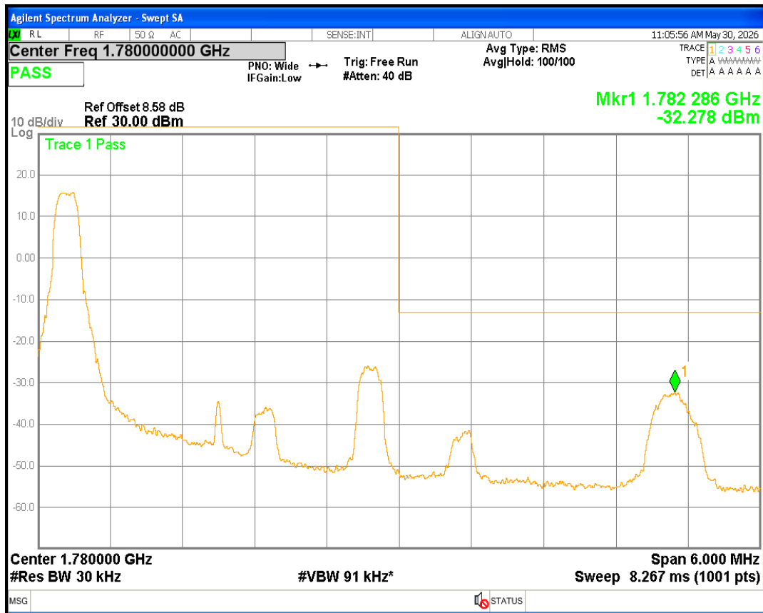
Band66 QPSK BW=3MHz Channel=131987 RB Size=15 Position=#0
