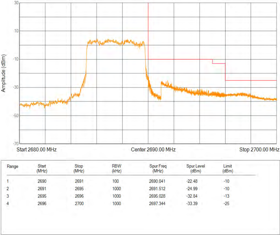
Band41 QPSK BW=10MHz Channel=39700 RB Size=1 Position=#0
