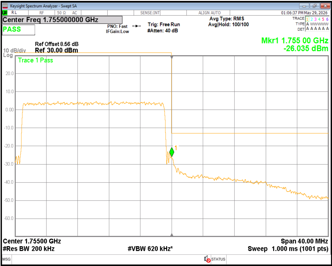
Band41 16QAM BW=5MHz Channel=39675 RB Size=1 Position=#0
