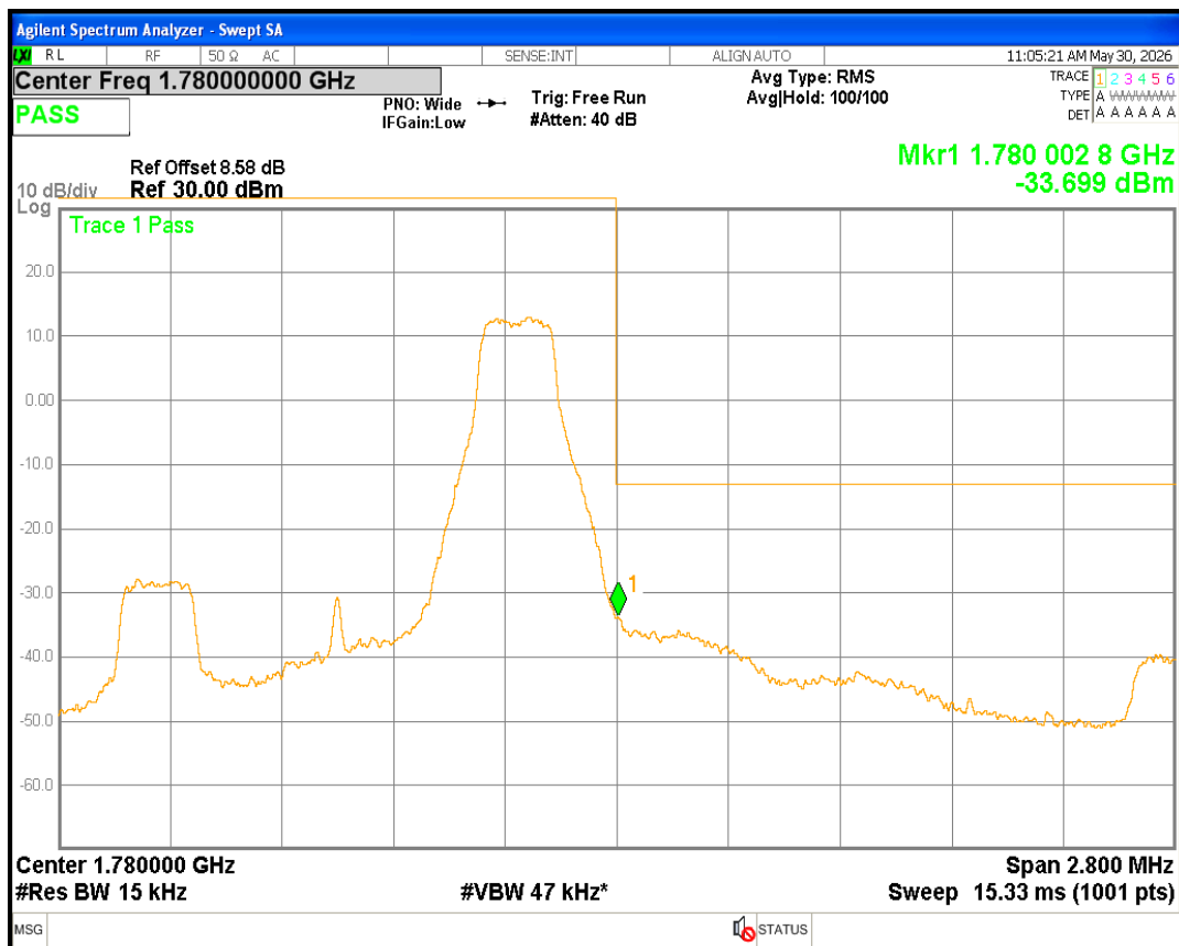
Band66 16QAM BW=1.4MHz Channel=132665 RB Size=6 Position=#0
