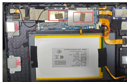
Apply conductive sponge on the motherboard shield for grounding.
