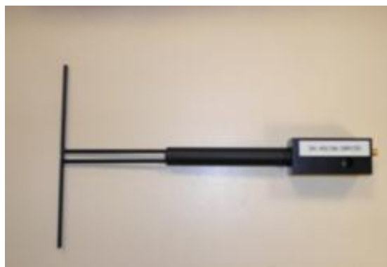
Figure 1 – MVG COMOSAR Validation Dipole
