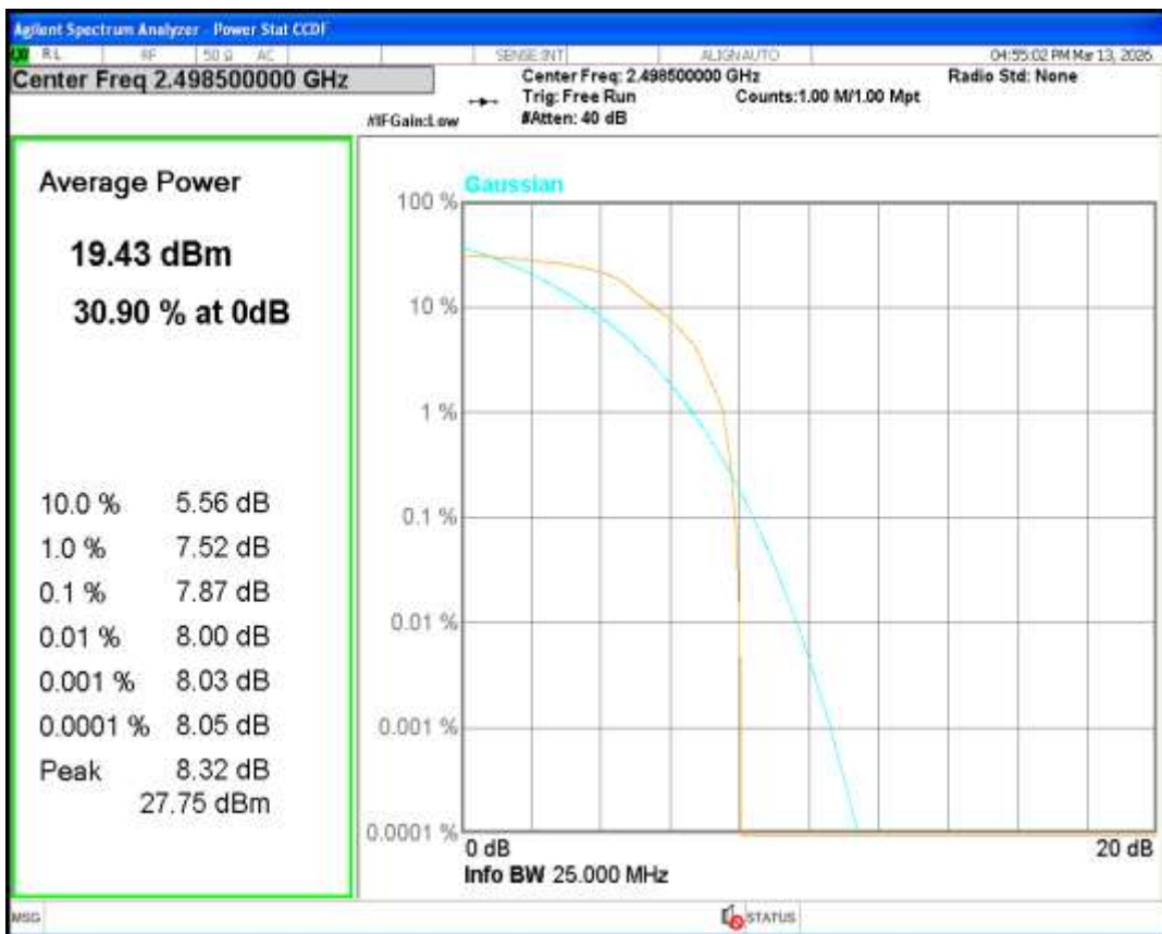
Band41 QPSK BW=5MHz Channel=40620 RB Size=1 Position=#0
