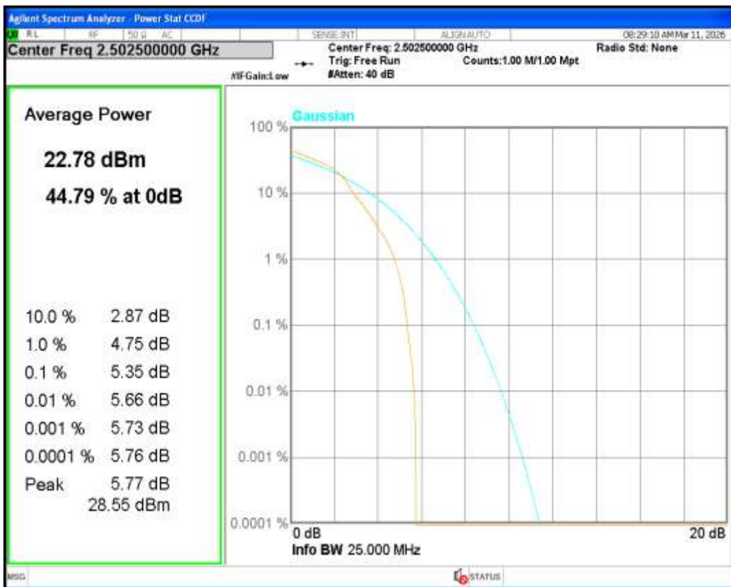
Band7 QPSK BW=15MHz Channel=20825 RB Size=1 Position=#0
