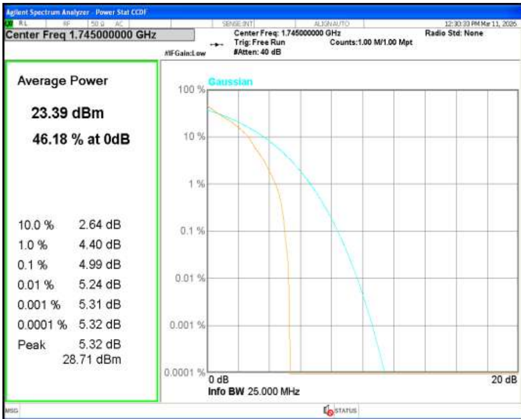
Band66 QPSK BW=10MHz Channel=132622 RB Size=1 Position=#0
