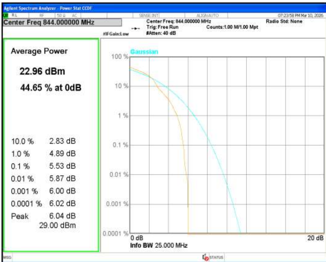
Band5 16QAM BW=3MHz Channel=20415 RB Size=1 Position=#0
