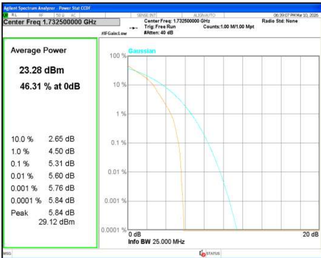
Band4 QPSK BW=1.4MHz Channel=20393 RB Size=1 Position=#0
