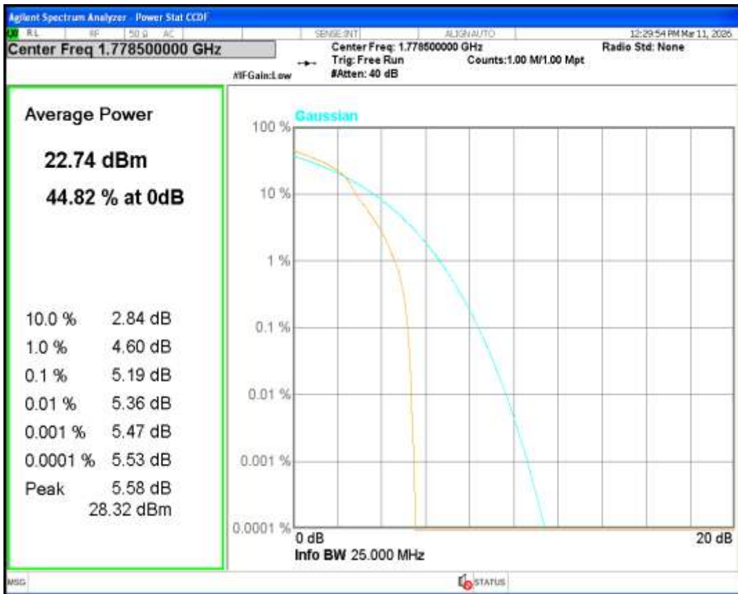
Band66 QPSK BW=1.4MHz Channel=132322 RB Size=1 Position=#0
