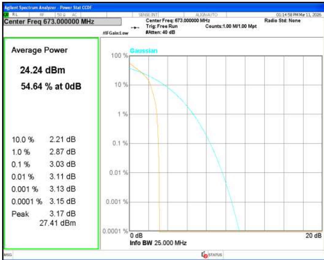
Band71 QPSK BW=20MHz Channel=133297 RB Size=1 Position=#0
