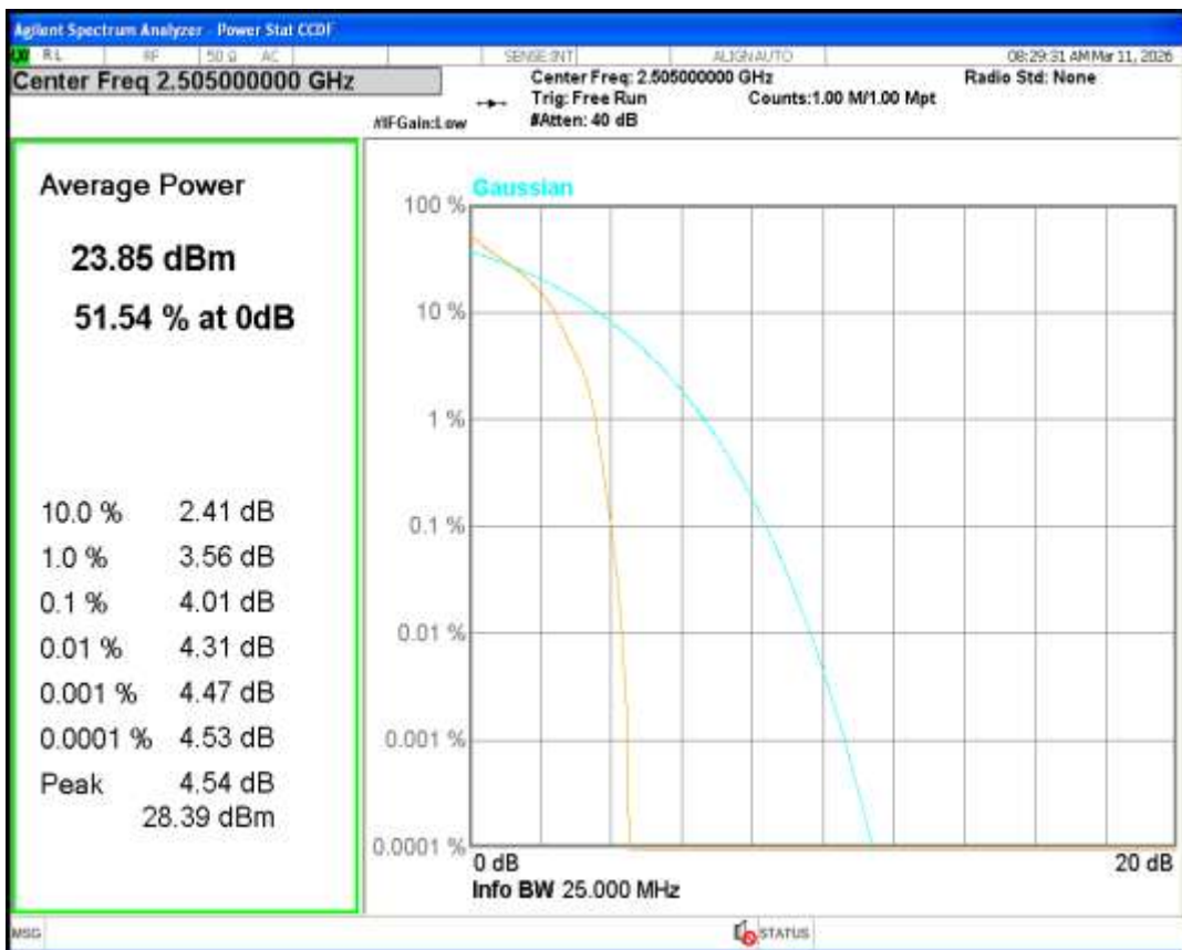
Band7 QPSK BW=15MHz Channel=21100 RB Size=1 Position=#0
