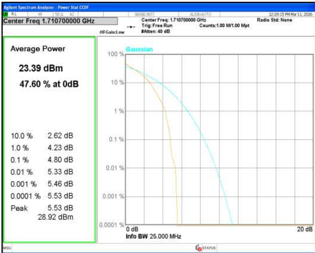
Band66 16QAM BW=5MHz Channel=132647 RB Size=1 Position=#0
