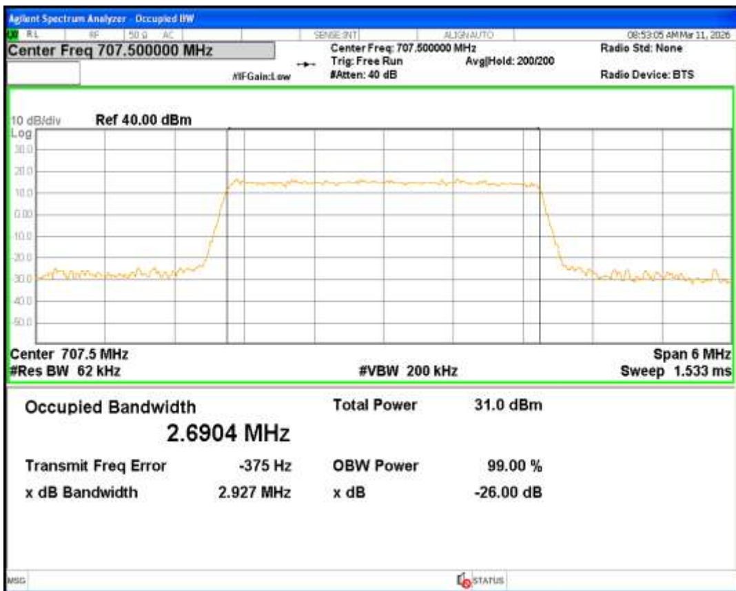
Band12 16QAM BW=3MHz Channel=23165 RB Size=15 Position=#0
