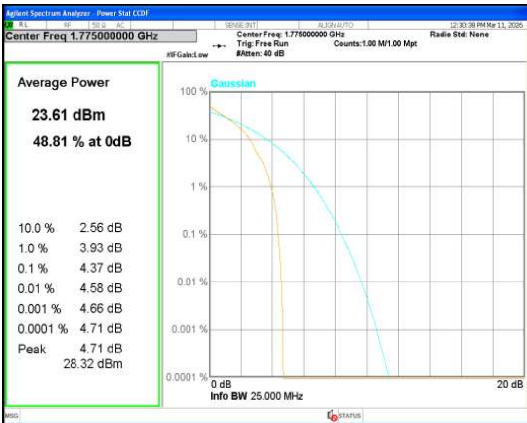
Band66 QPSK BW=15MHz Channel=132047 RB Size=1 Position=#0
