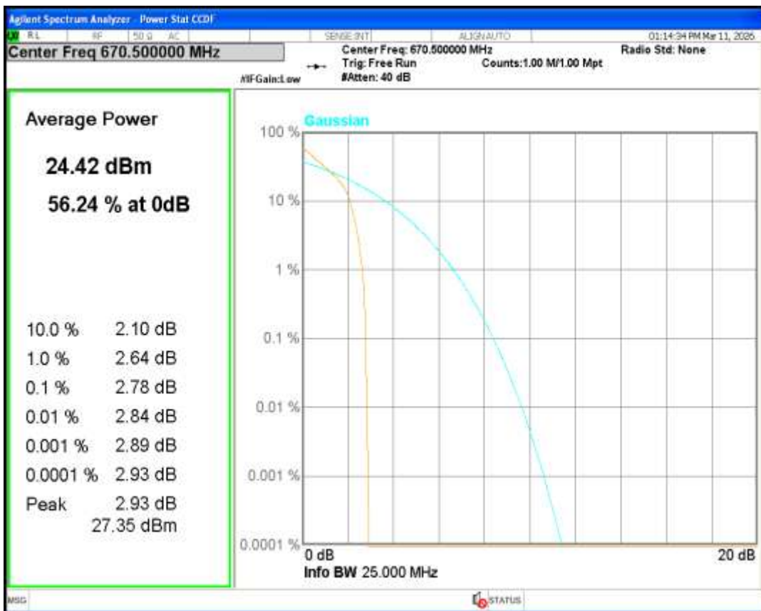
Band71 QPSK BW=15MHz Channel=133297 RB Size=1 Position=#0
