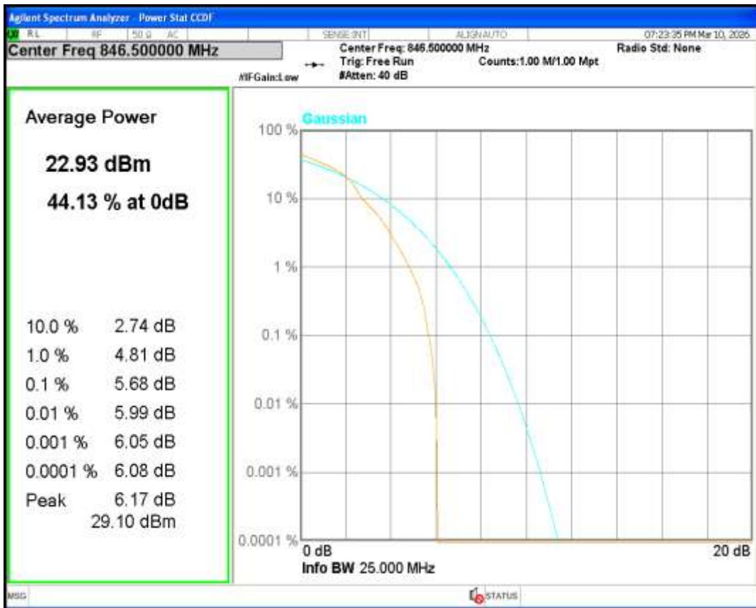
Band5 16QAM BW=5MHz Channel=20525 RB Size=1 Position=#0
