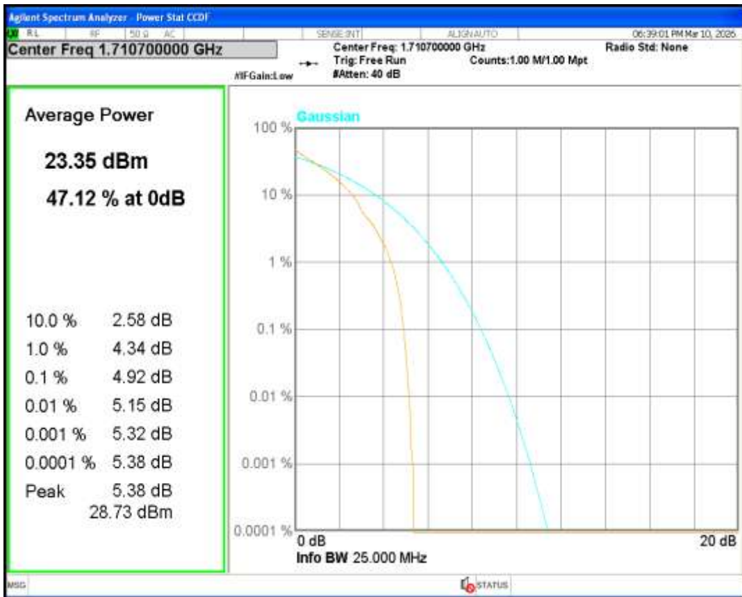
Band4 QPSK BW=1.4MHz Channel=20175 RB Size=1 Position=#0
