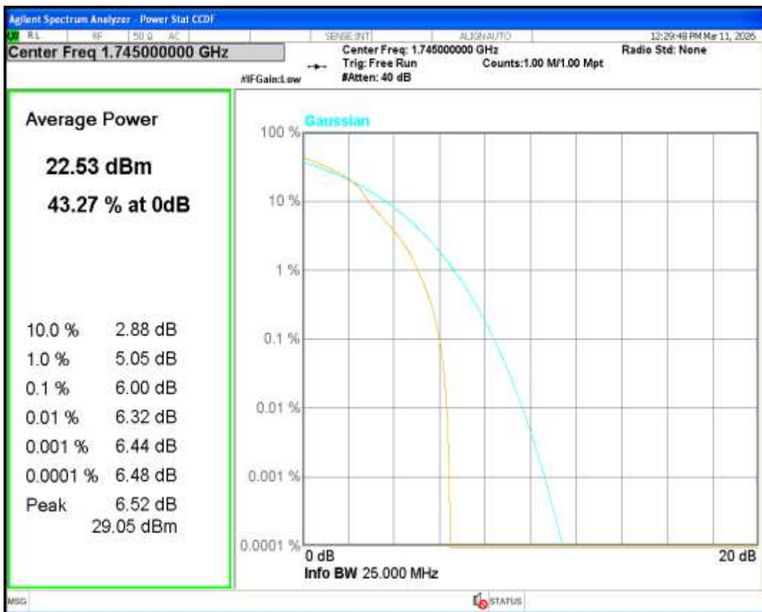
Band66 16QAM BW=3MHz Channel=132657 RB Size=1 Position=#0
