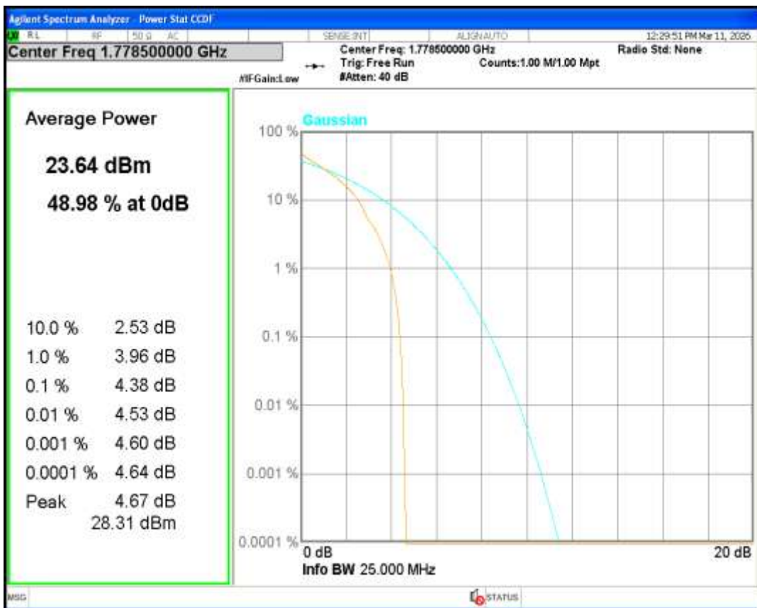
Band66 QPSK BW=5MHz Channel=131997 RB Size=1 Position=#0
