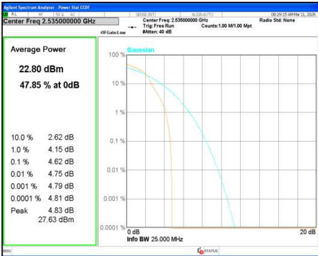
Band7 QPSK BW=10MHz Channel=20800 RB Size=1 Position=#0
