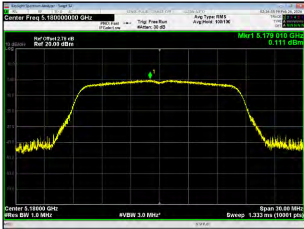
(802.11a) PSD plot on channel 40
