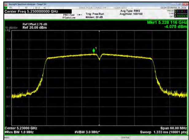
(802.11n40) PSD plot on channel 46
