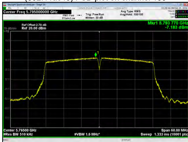
(802.11ac40) PSD plot on channel 159
