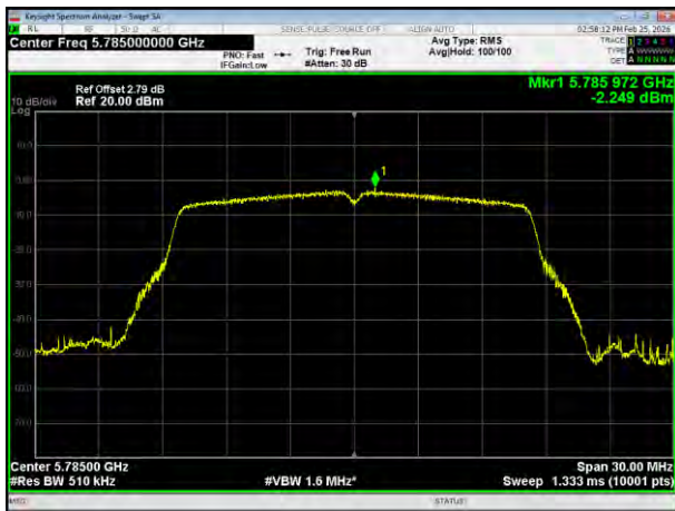
(802.11a) PSD plot on channel 157
