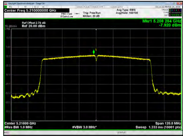
(802.11ac80) PSD plot on channel 42
