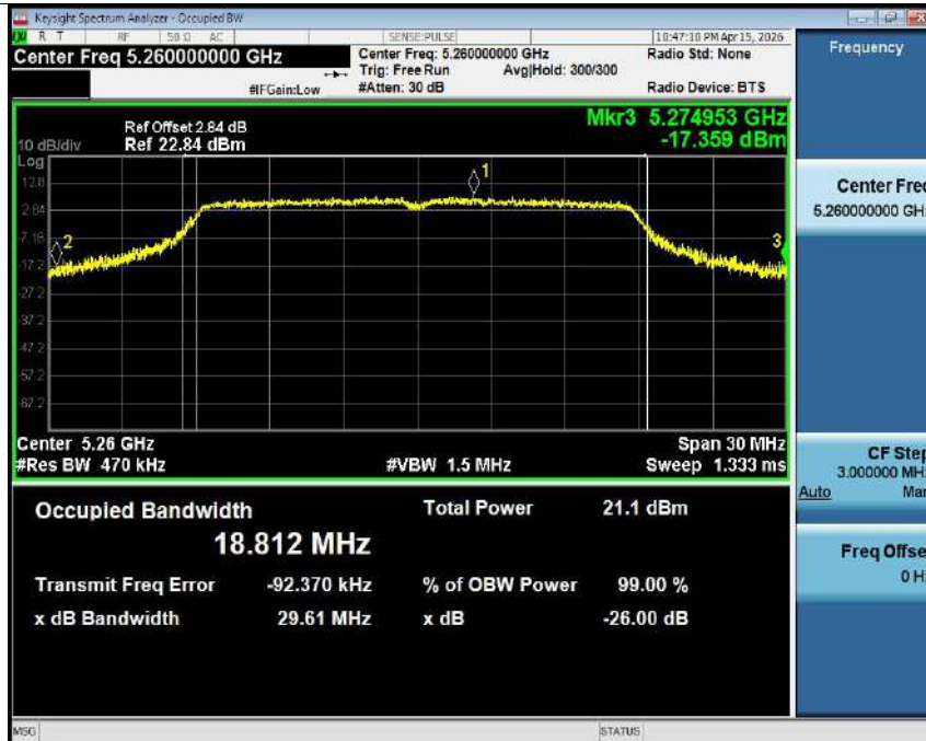
-26dB Bandwidth NVNT ac20 5260MHz Ant1
