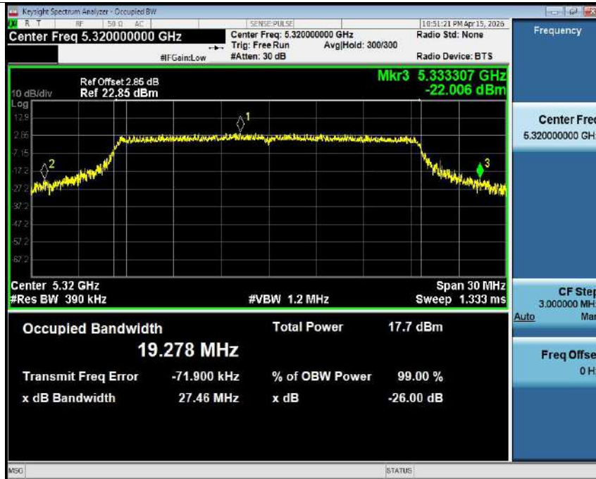
-26dB Bandwidth NVNT ax20 5320MHz Ant1
