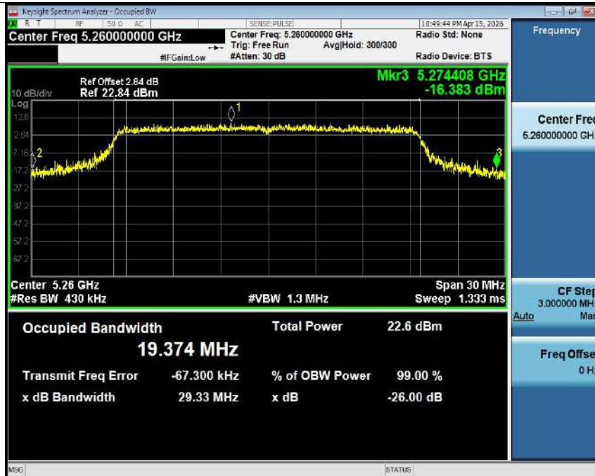
-26dB Bandwidth NVNT ax20 5260MHz Ant1
