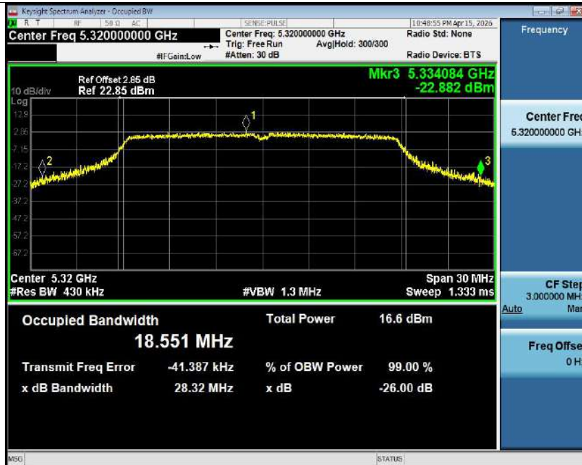
-26dB Bandwidth NVNT ac20 5320MHz Ant1
