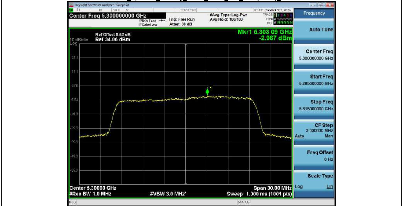
Power Spectral Density_NVNT_ANT1_802_11ax(HE20)_5300
