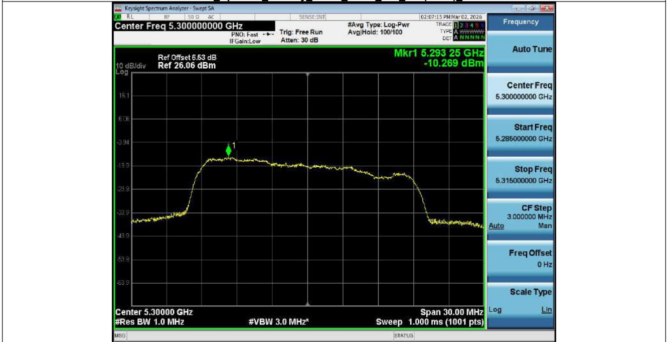
Power Spectral Density NVNT ANT1 802_11n(HT20)_5300
