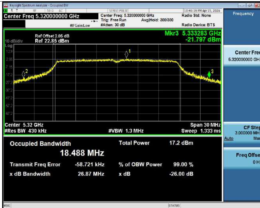
-26dB Bandwidth NVNT n20 5320MHz Ant1
