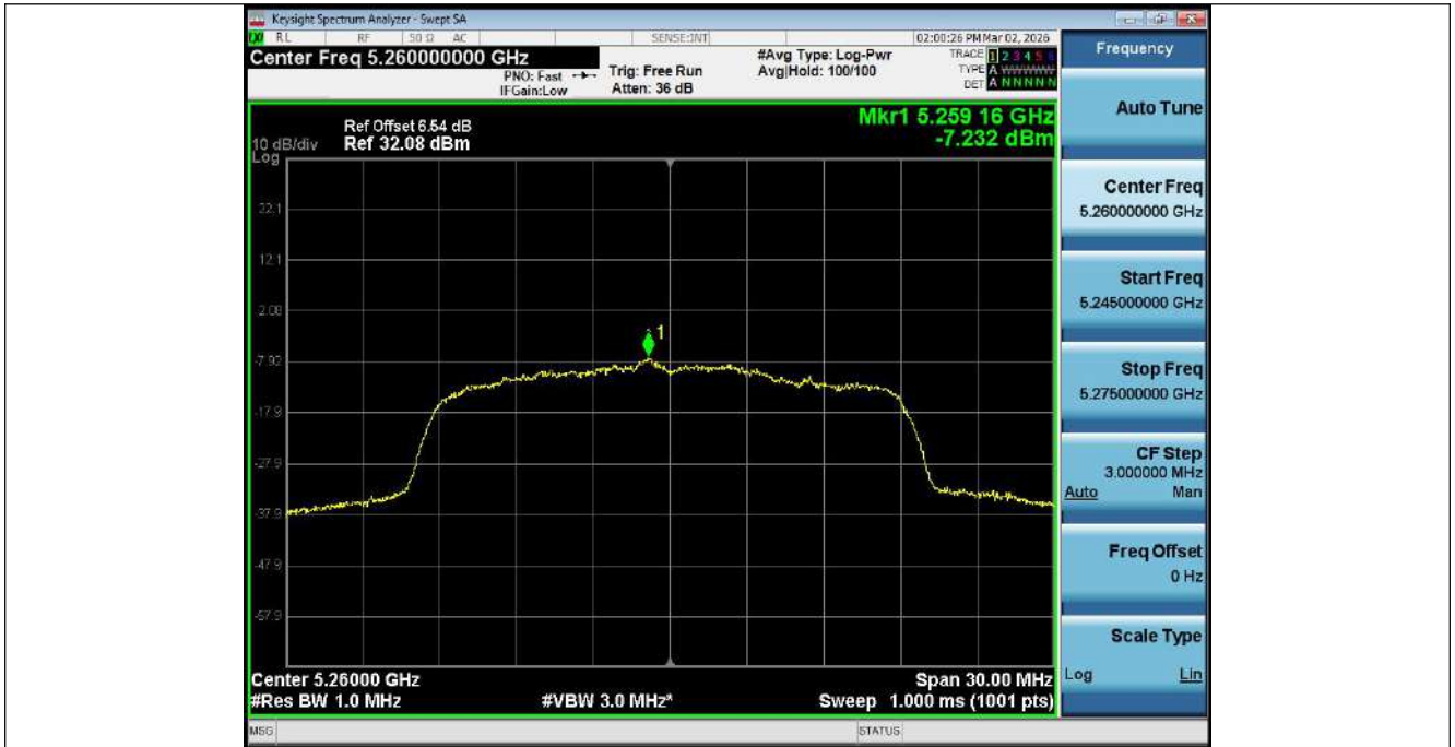
Power Spectral Density NVNT ANT1 802_11n(HT20)_5300
