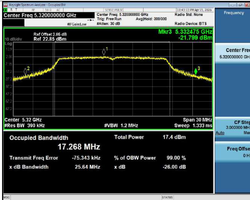
-26dB Bandwidth NVNT a 5320MHz Ant1
