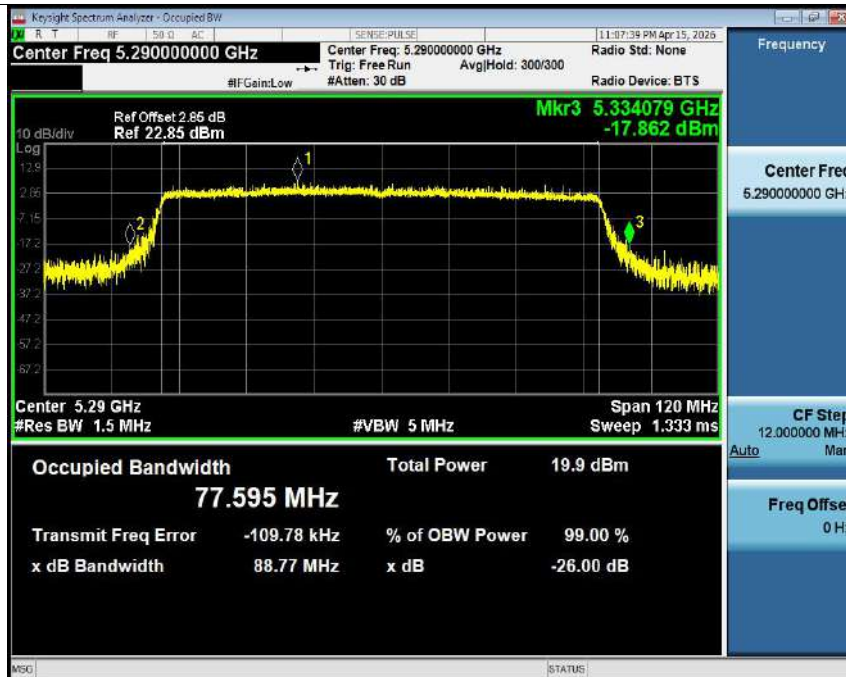
-26dB Bandwidth NVNT ax80 5290MHz Ant1
