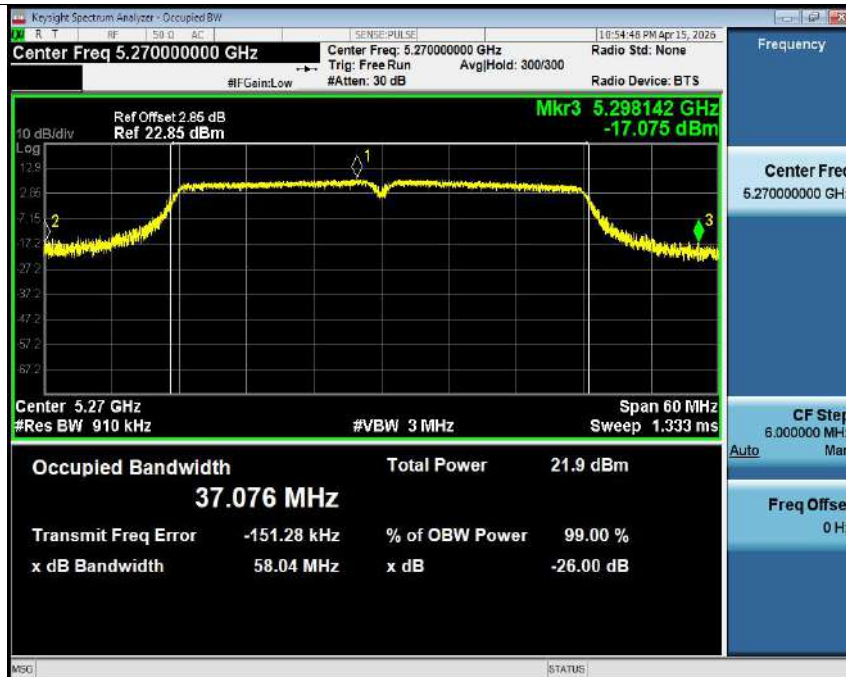
-26dB Bandwidth NVNT ac40 5270MHz Ant1
