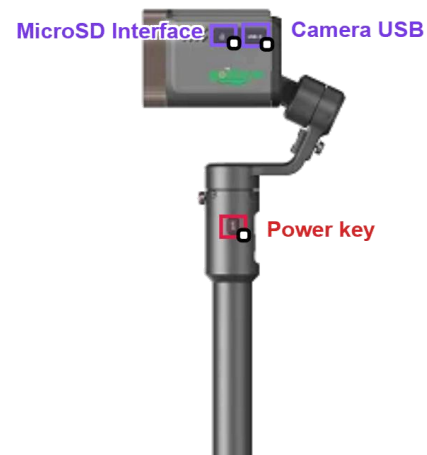
Right: microSD + USB + Power key
