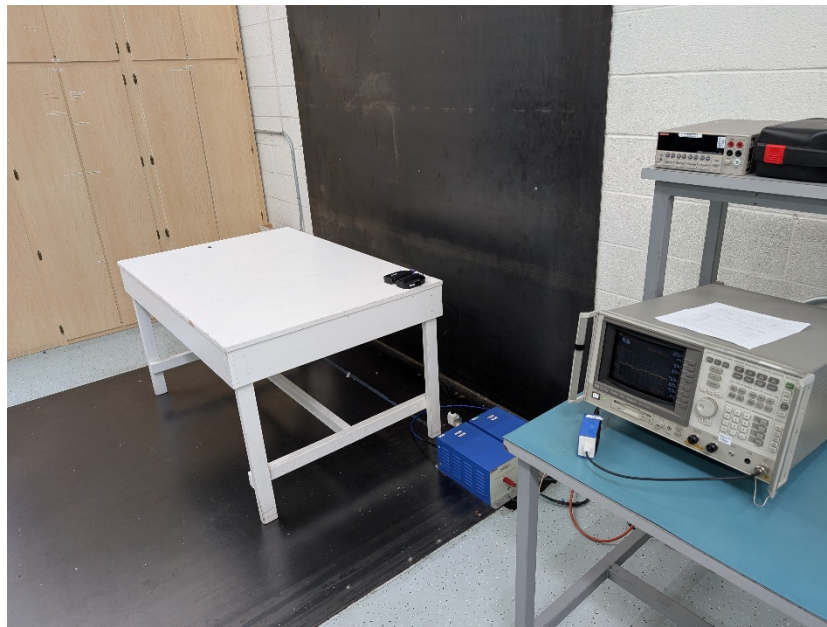
AC Power line Conducted Test Setup 1
