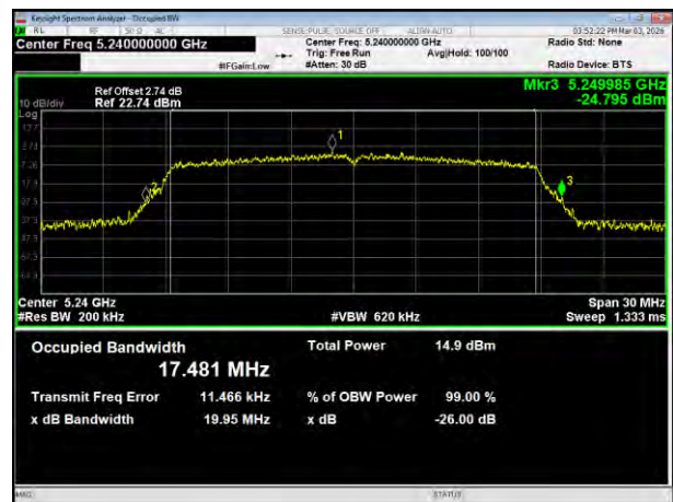
(802.11 n20) plot on channel 48
