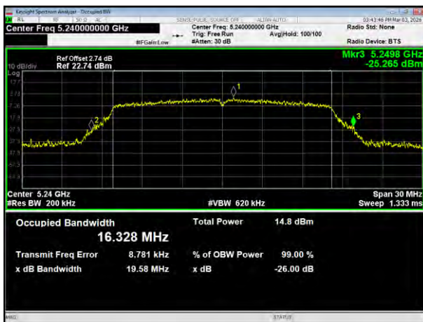
(802.11a) plot on channel 48
