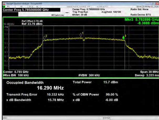
(802.11a) plot on channel 165
