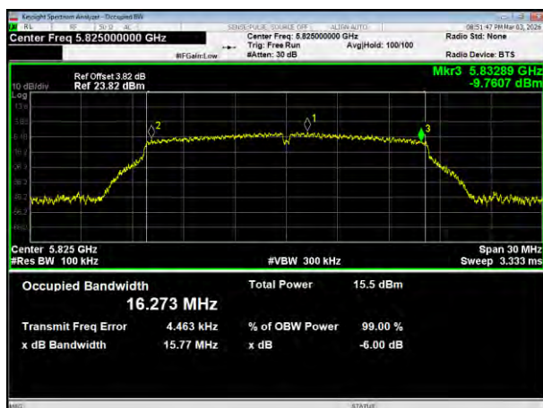
(802.11a) plot on channel 165
