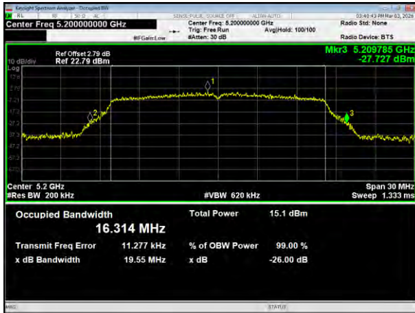
(802.11a) plot on channel 48
