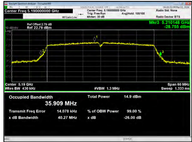
(802.11 n40) plot on channel 46
