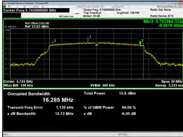
(802.11a) plot on channel 157
