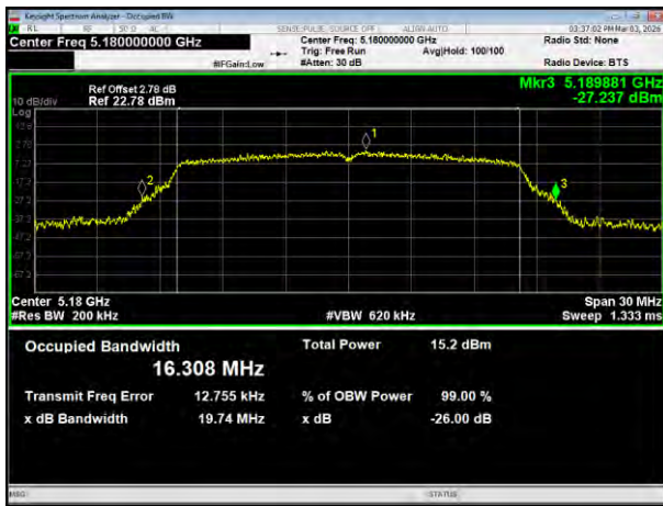
(802.11a) plot on channel 40
