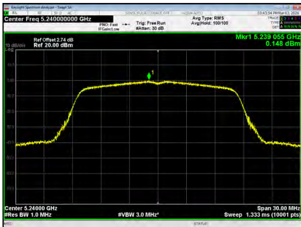
(802.11a) PSD plot on channel 48
