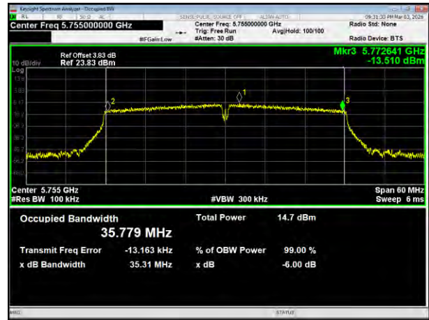
(802.11 n40) plot on channel 159
