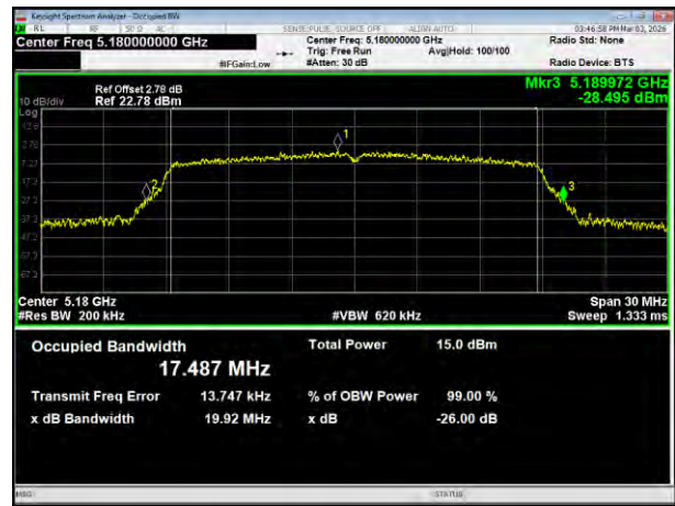
(802.11 n20) plot on channel 40
