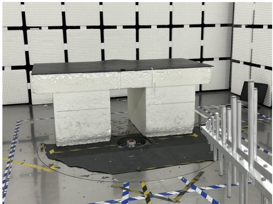
Radiation Emission Test Setup (30MHz to 1GHz)
