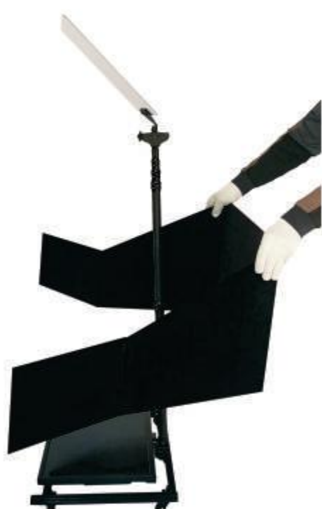
7 Take out the foldable barndoors open it and place it as picture
