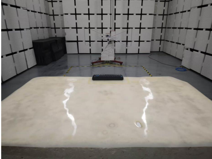
Set-up for Radiated Spurious Emission, Above 1GHz
