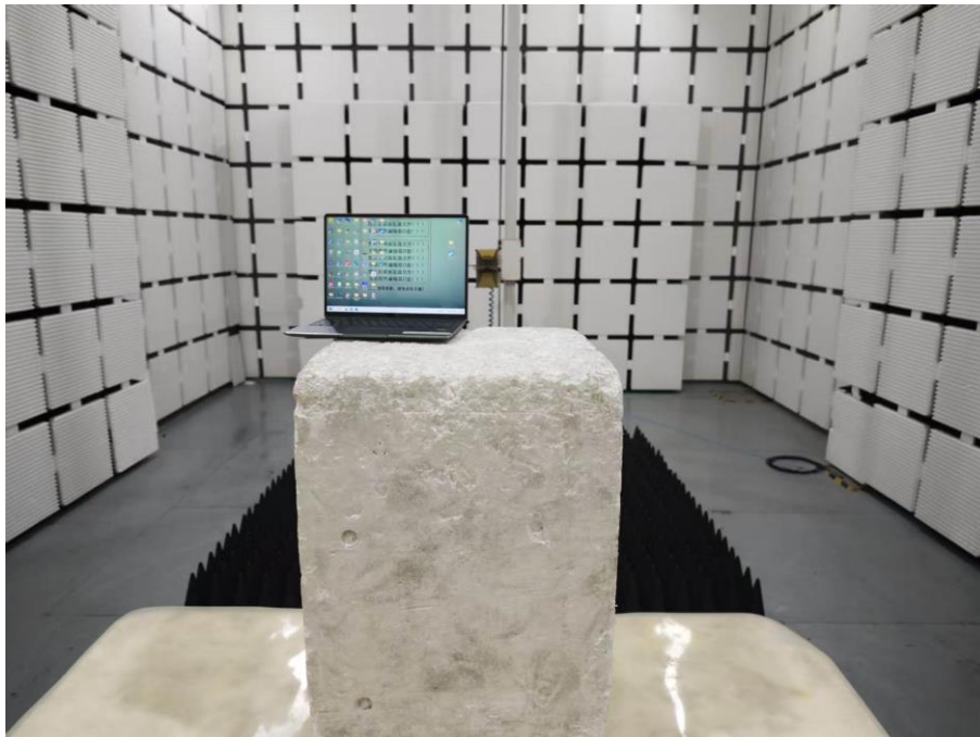
Set-up for Radiated Spurious Emission, Above 1GHz
