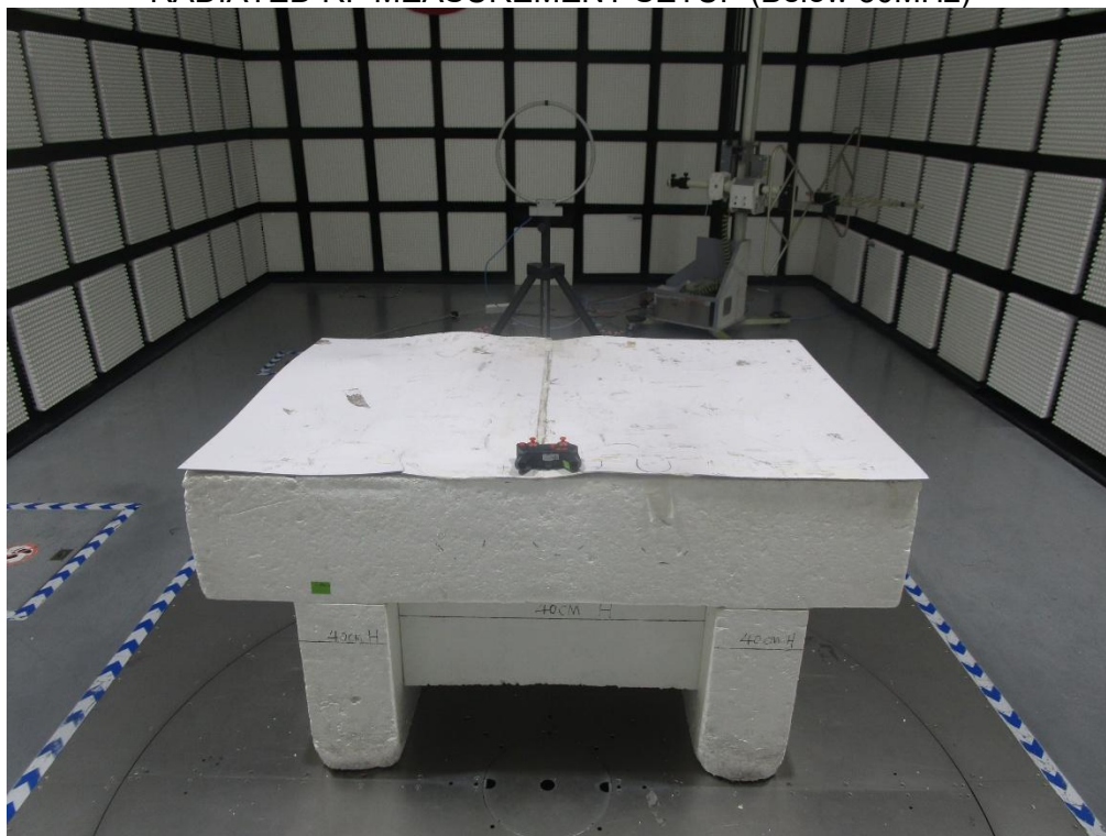
RADIATED RF MEASUREMENT SETUP (Below 30MHz)
