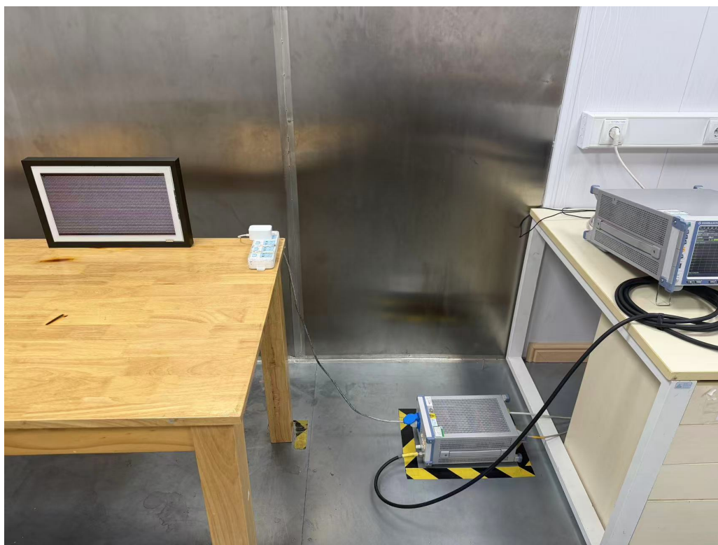
Photograph 3: Set-up photo for AC conducted emissions
