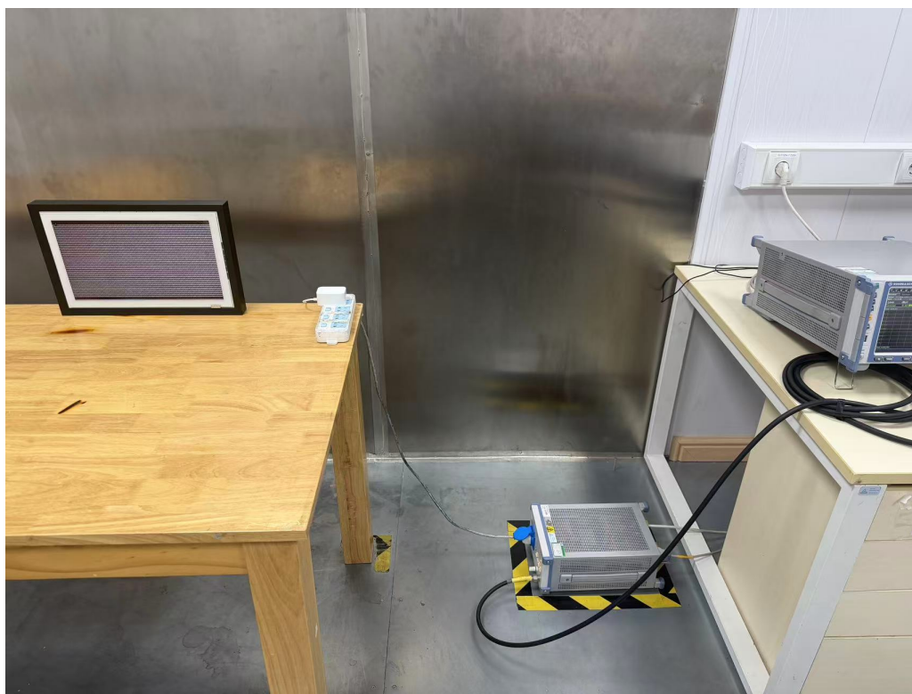
Photograph 3: Set-up photo for AC conducted emissions
