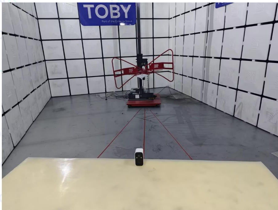
Photo of Setup for Radiated Emission (30MHz~1GHz)
