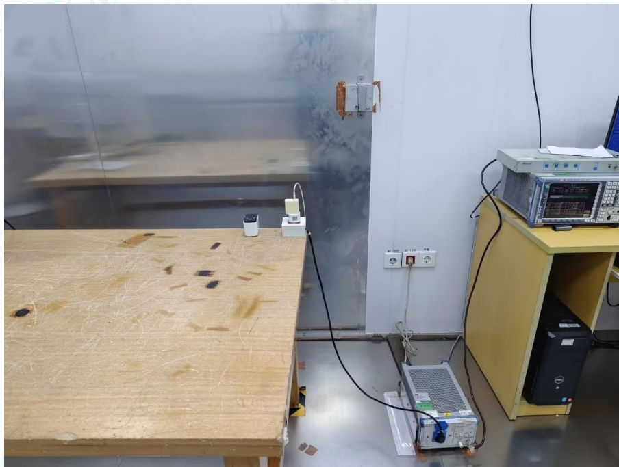
Photo of Setup for Radiated Emission (30MHz~1GHz)
