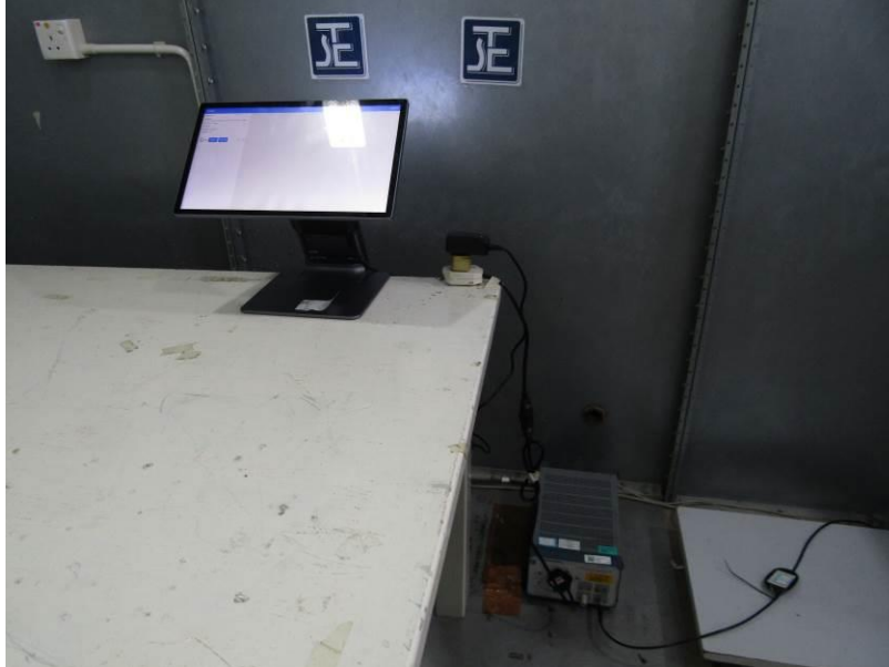
Measurement of Conducted Emission Test Set Up
