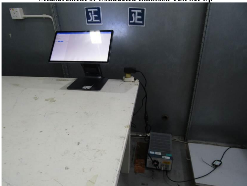
Measurement of Conducted Emission Test Set Up
