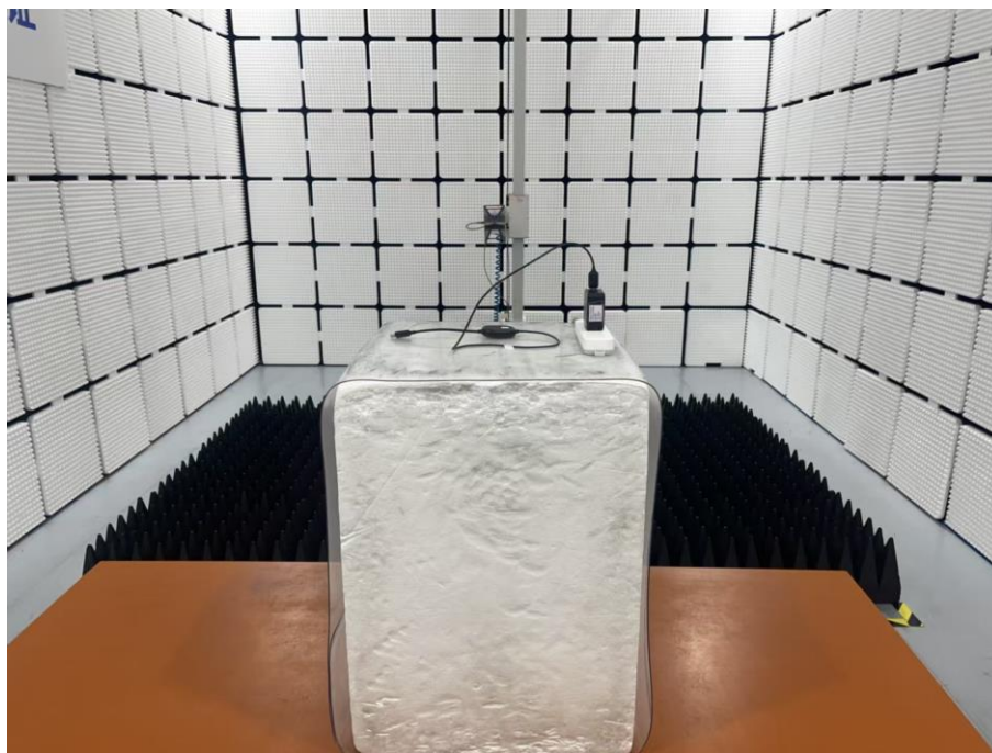
Radiated Emission Above 1GHz
