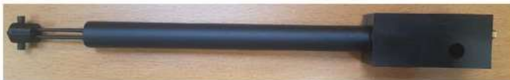
Figure 1 – MVG COMOSAR Validation Dipole
