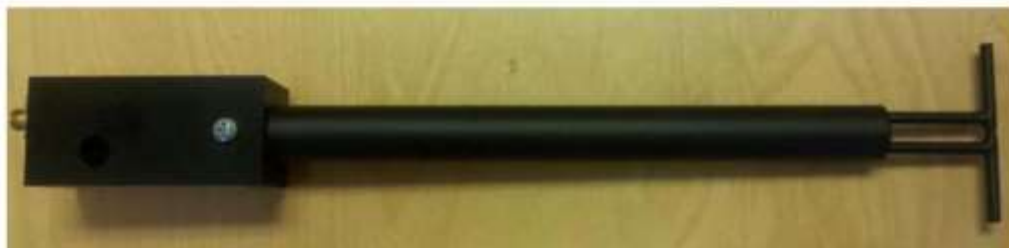
Figure 1 – MVG COMOSAR Validation Dipole
