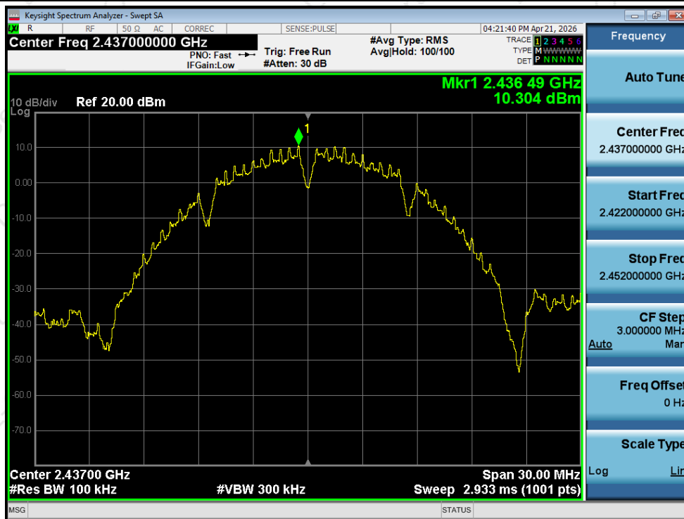
Tx. Spurious NVNT b 2437MHz Ant1 Ref
