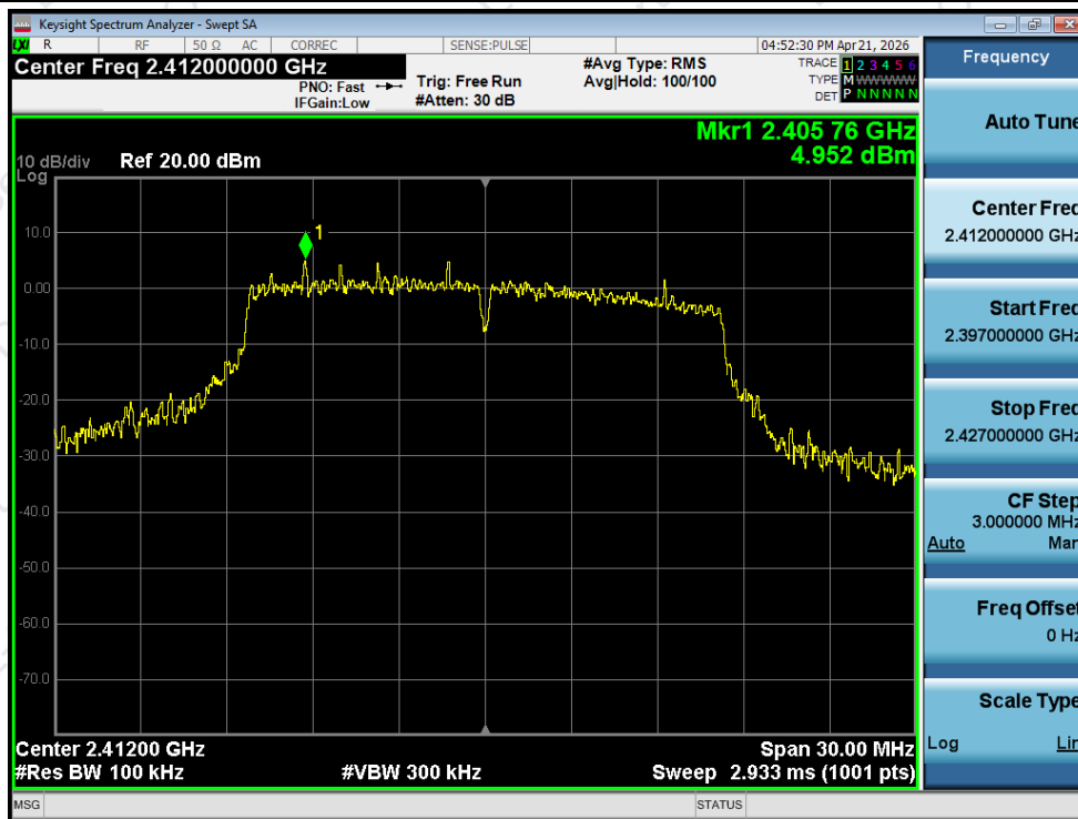
Tx. Spurious NVNT g 2412MHz Ant1 Ref
