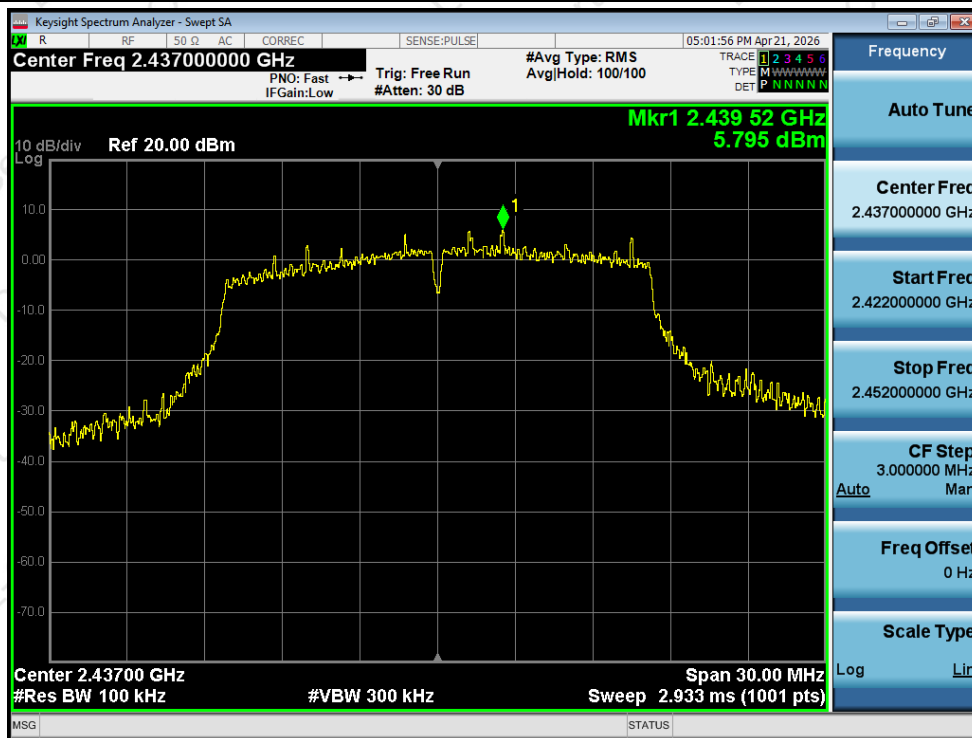
Tx. Spurious NVNT g 2437MHz Ant1 Ref
