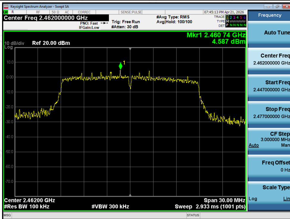
Tx. Spurious NVNT n20 2462MHz Ant1 Ref
