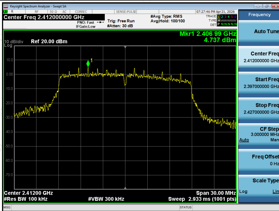
Tx. Spurious NVNT n20 2412MHz Ant1 Ref
