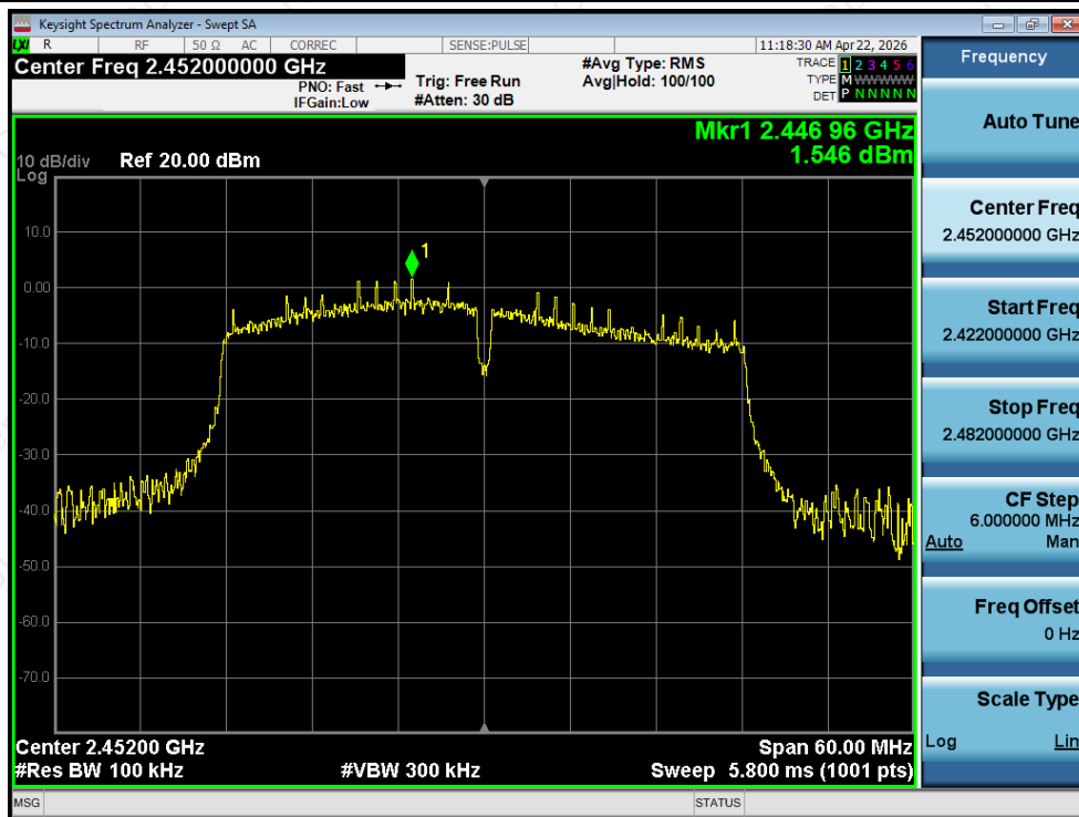
Tx. Spurious NVNT n40 2452MHz Ant1 Ref
