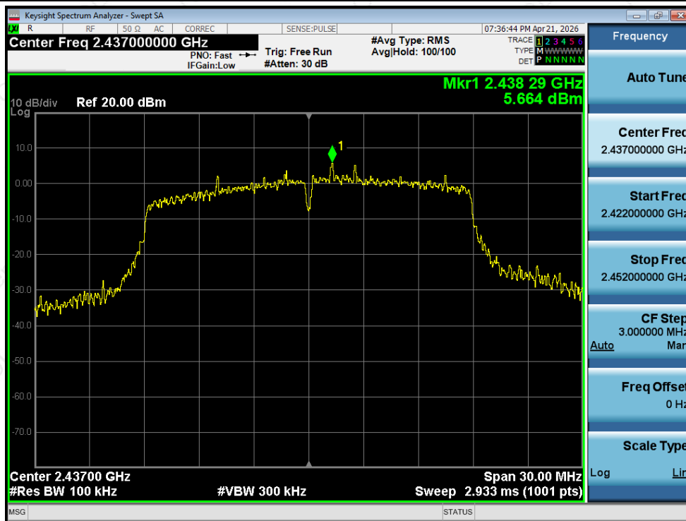
Tx. Spurious NVNT n20 2437MHz Ant1 Ref
